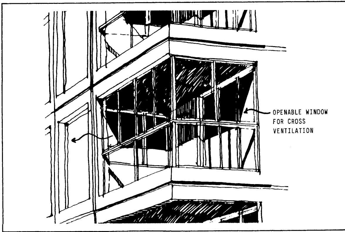
Figure 7. Example of an Encouraged Balcony Enclosure that Retains the Building's Exterior Wall Glazing (for Smoke Isolation) between the Main Living Area and Enclosed Balcony
