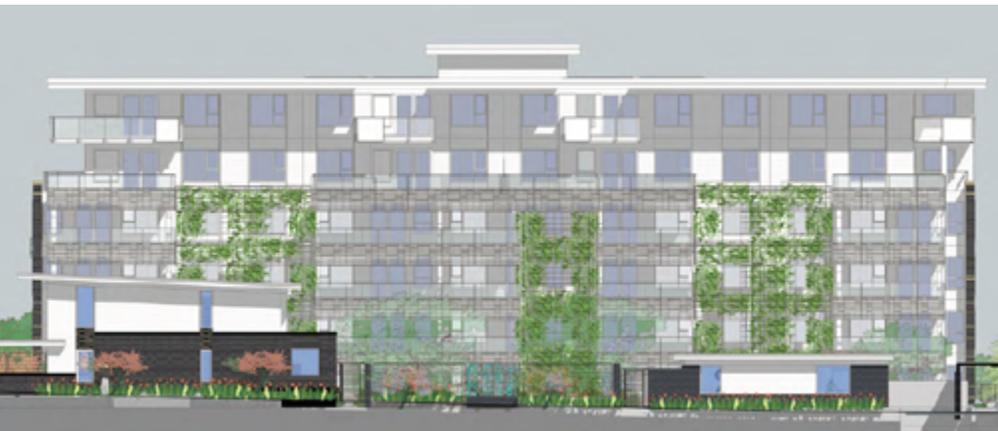
Fig. 16 | Laneway facade designed with lighter framework of columns and beams
