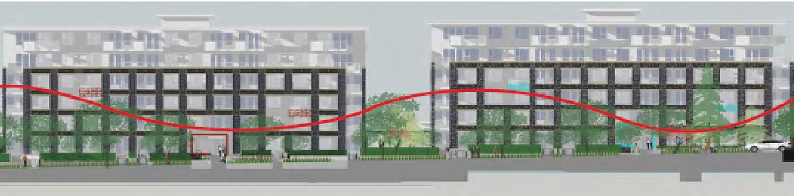
Fig. 11 | Two 2-storey openings have been introduced at different floor levels of the brick screen walls to create a rhythmic modulation reinforcing the layering concept of the facade
