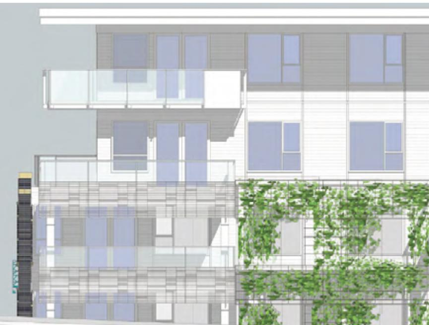
Fig. 18 | Balconies at the rear of the building designed as a light structure to provide vertical shading from the low western sun
