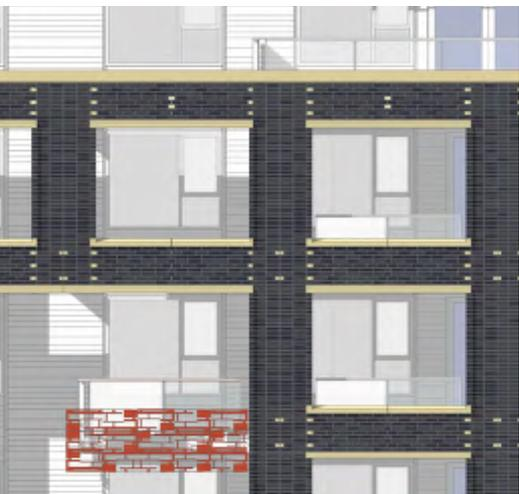
Fig. 8 | Masonry of the south building using a "stitched" accent pattern
