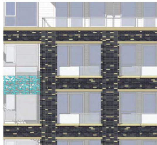
Fig. 7 | Masonry of the north building using a random accent pattern
