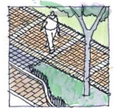
Primary City sidewalk with concrete unit paving, granite set boulevard and shrub planting or raingardens at corner and midblock bulges.
