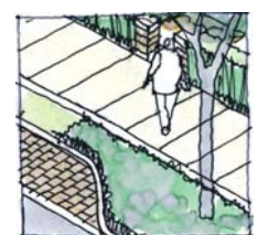
Secondary City sidewalk with broom finished concrete, lawn boulevard, and shrub planting or raingardens at corner and midblock bulges.
