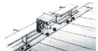
F: Deck bullrail with lighting
