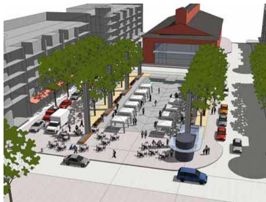
In summer, vertical solar elements along the length of the plaza would utilize solar energy to operate a water feature in the plaza, using recirculating rainwater stored in the cistern beneath.
