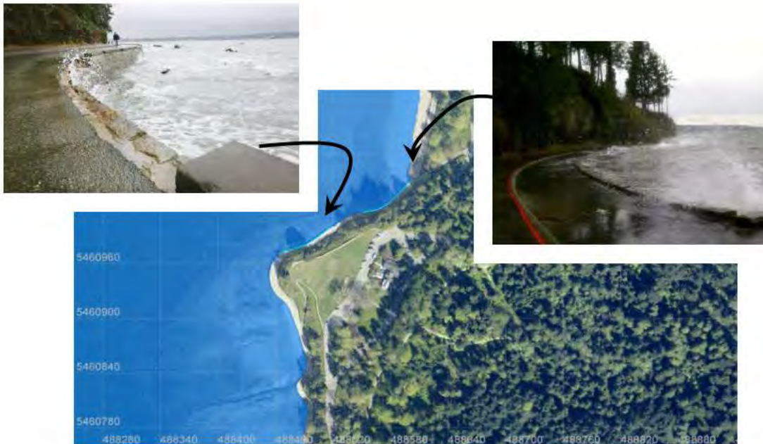
Figure 19. Comparison of observed and simulated flood extents along Stanley Park seawall near the Teahouse Restaurant for December 17, 2012.
