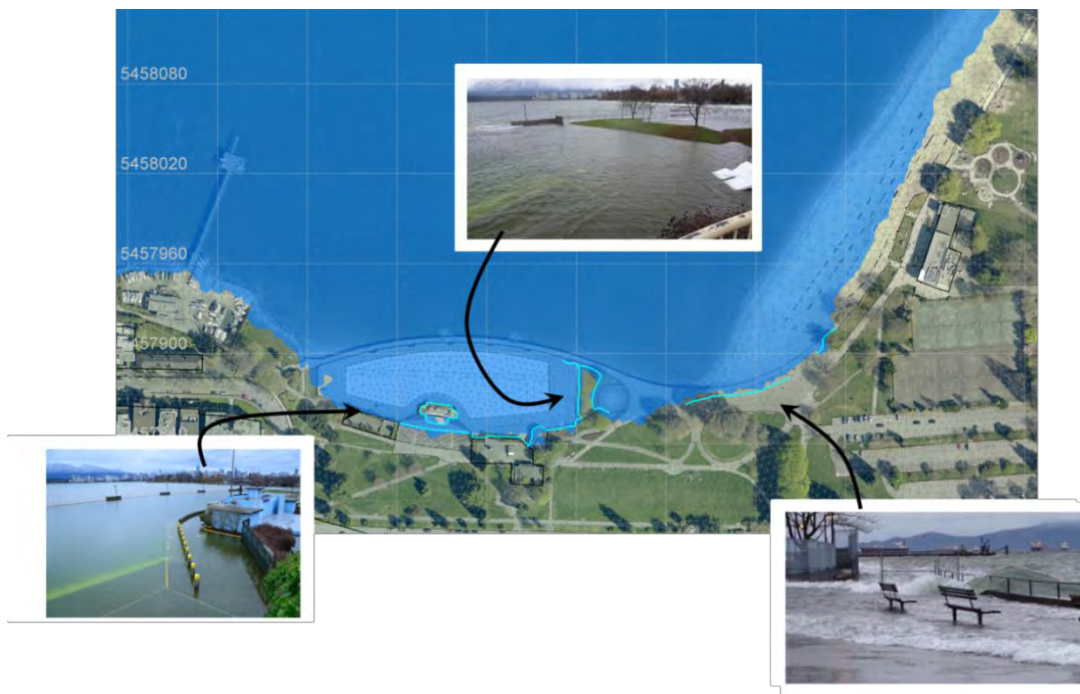
Figure 13. Comparison of observed and simulated flood extents at Kitsilano Pool and Beach for December 17, 2012.
