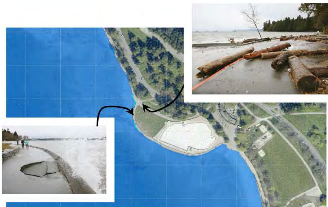
Figure 18. Comparison of observed and simulated flood extents along the seawall near Second Beach Pool for December 17, 2012.
