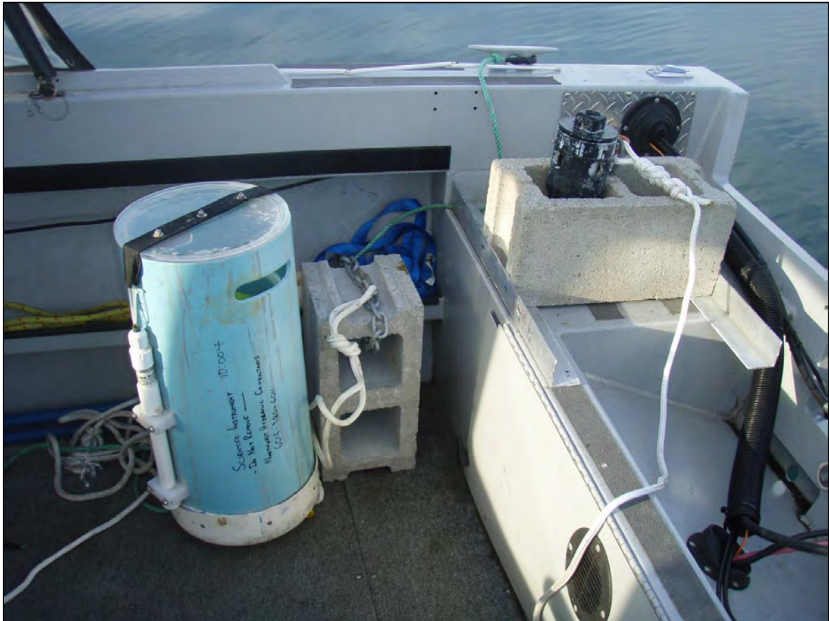
Figure 2. Wave sensor (black tube at right), with cinder block anchors and timed float (blue tube at left).
