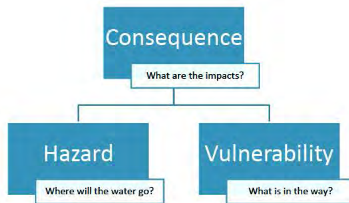
Figure 9: Flood consequence as a function of hazard and vulnerability
