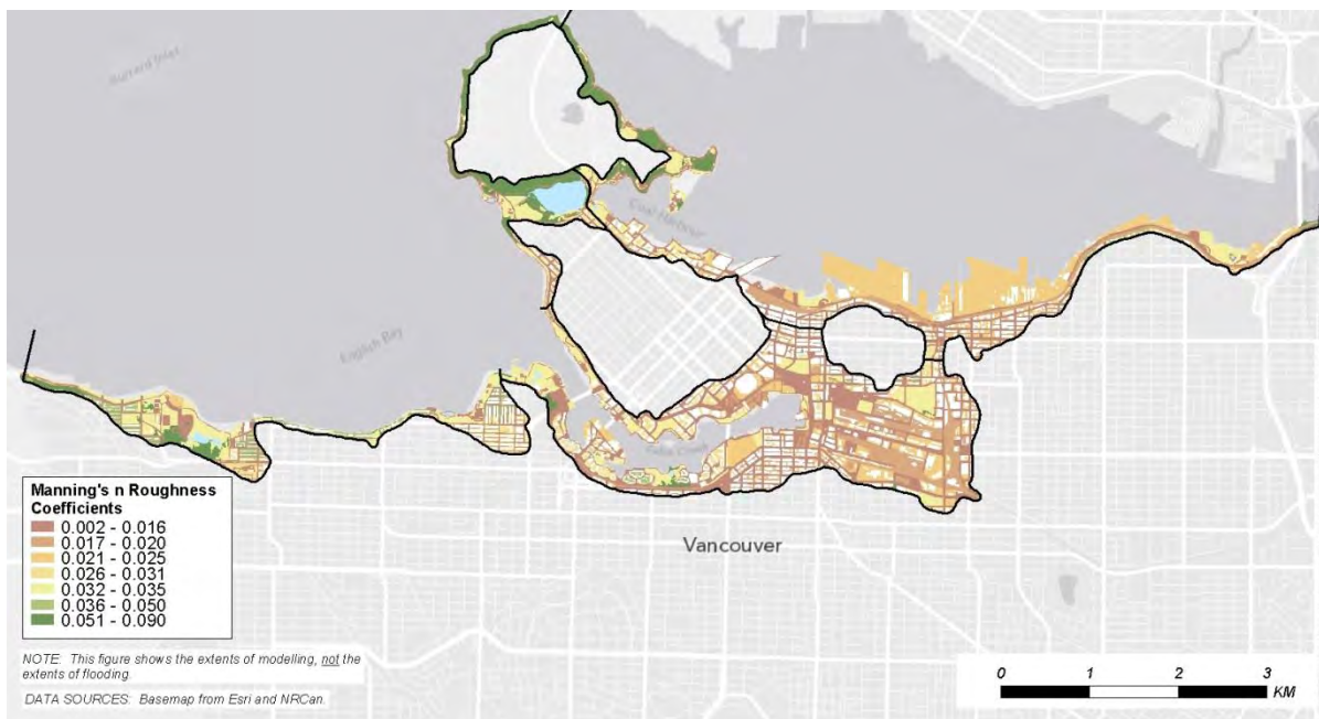
Figure 11. Roughness coefficients assigned to the mesh based on landuse classes.
