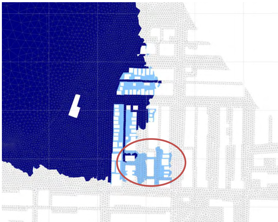
Figure 23. Comparison of modelled flood extents for mesh with generalized buildings (dark blue) and mesh with original building footprints (light blue).
