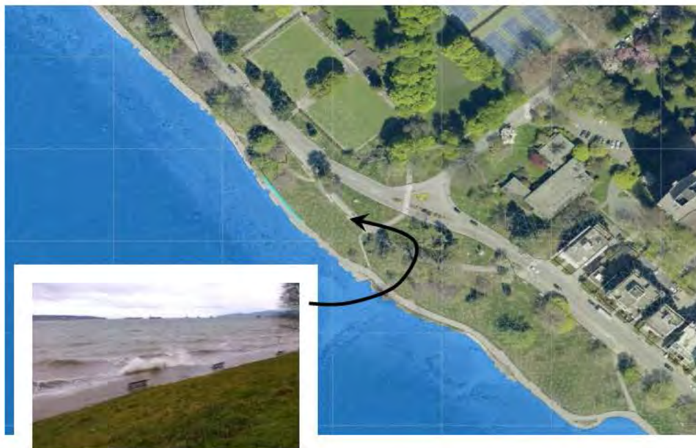
Figure 17. Comparison of observed and simulated flood extents along the seawall near Stanley Park Pitch and Putt for December 17, 2012.
