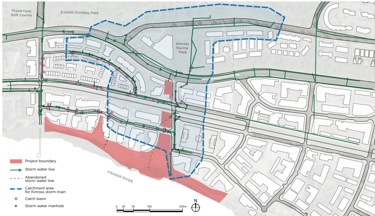
Site Drainage and Kinross Storm Water Catchment Area
