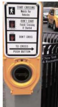
Accessible Pedestrian Signals 4 locations in pilot
