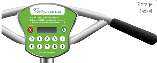
The Smoove "Brain" is a waterproof control box located on the handlebars. Members simply tap their card to unlock a bike. Casual riders enter their assigned PIN on the keypad to unlock the bike.
