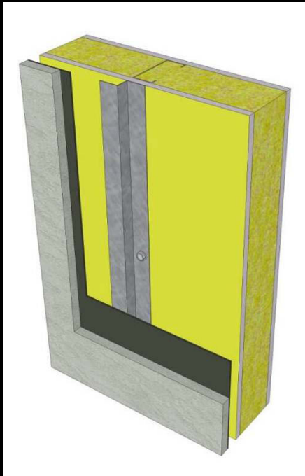
R-7.9 Cavity insulation between framing at 16" OC
