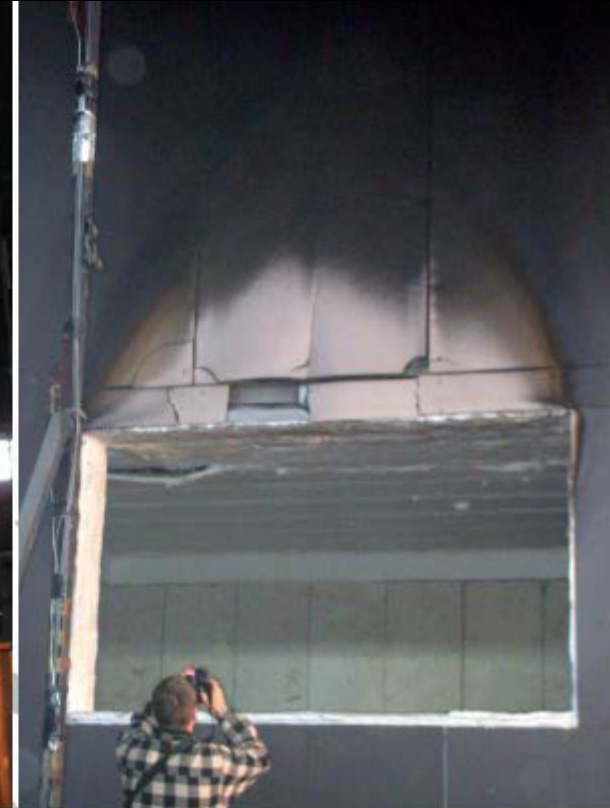
Figure 18: Photographs of the SWISSPEARL Exterior Wall Cladding CAN/ULC-S134 Test (a) Pre-burn wall assembly, (b) post-burn wall assembly damage.
