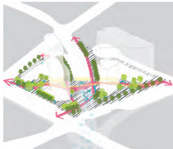
Figure 13 The Area 5B development schematic showing circulation, tree program, flooring and lighting strategies. Image by PFS Studio.
