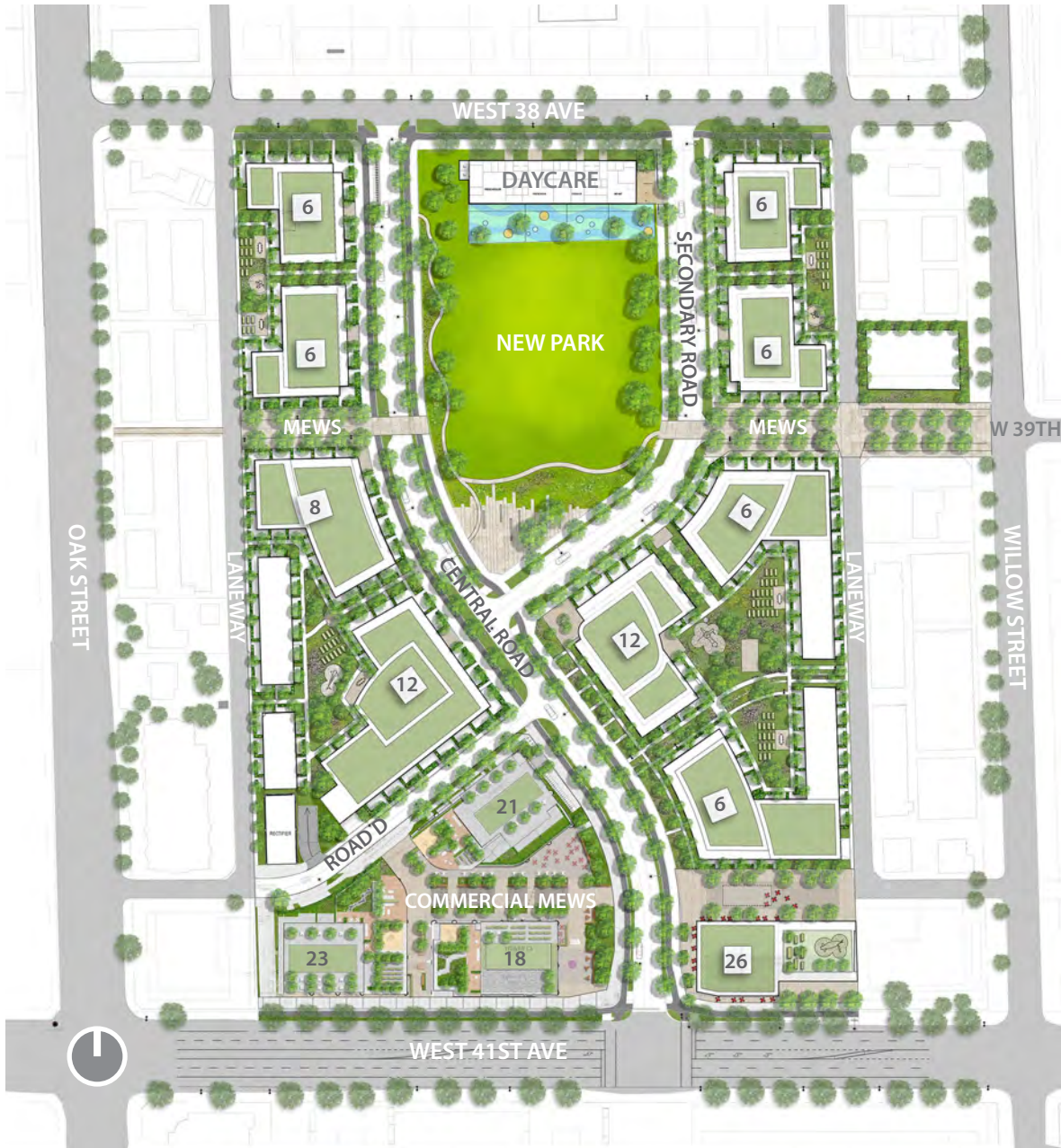
Figure 07 SITE PLAN for the Grosvenor Mayfair West Master Plan, the number labels on each building indicate the number of storeys
