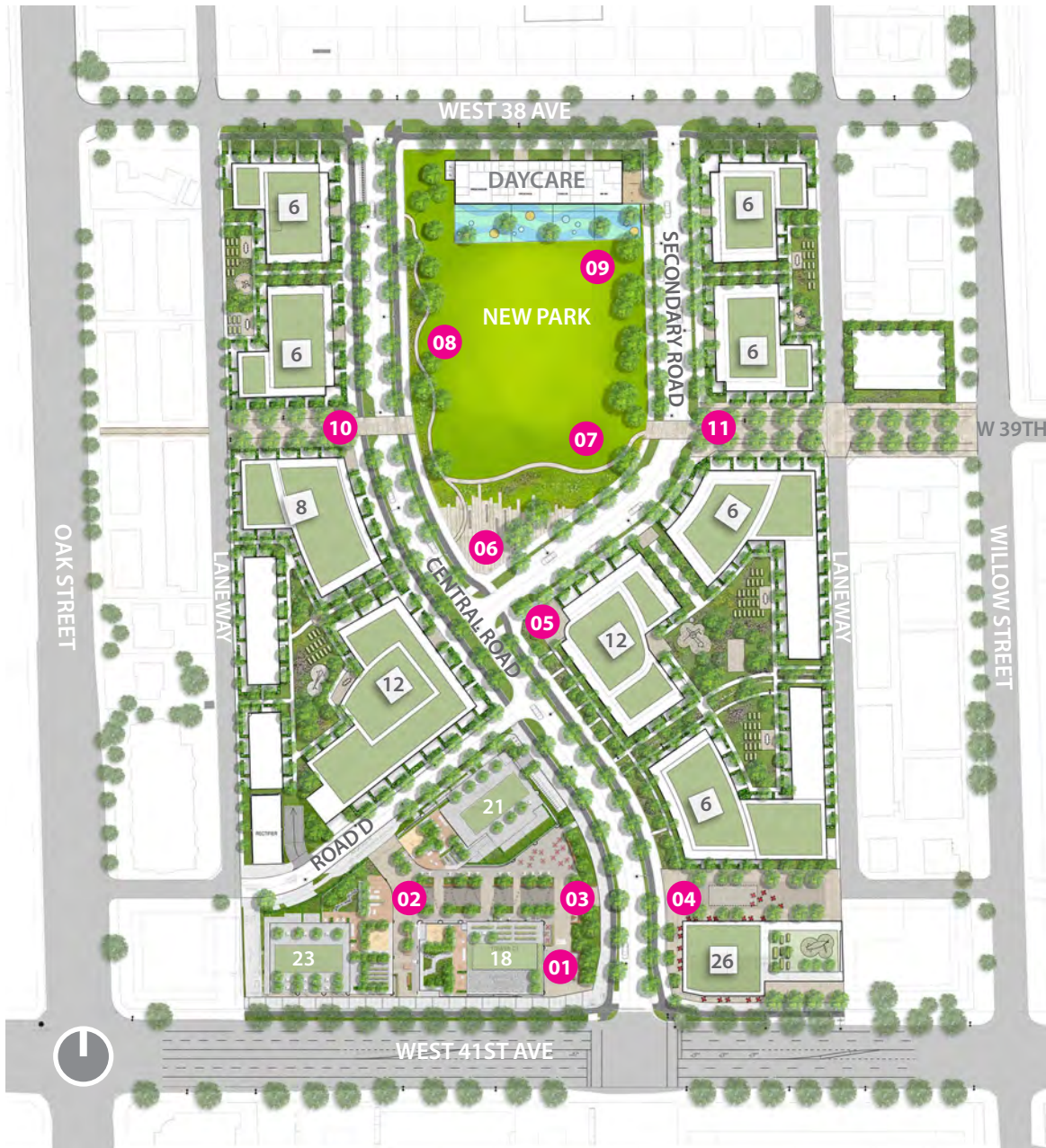
Figure 09 SITE PLAN for the Mayfair West Master Plan showing the potential art sites throughout the project designed by the circular markers, the number on each building refers to its number of storeys; rendered site plan by PFS Studio
