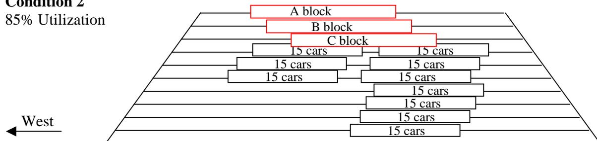
There are other effects of high levels of capacity utilization within a yard. In a yard where two engines work simultaneously, the extra moves that have to be made often conflict with the second engine's work. The more extra moves each engine has to make, the more opportunities exist for them to conflict with each other. This leads to further inefficiencies and potential service delays within the yard, which require additional time, effort and cost.
