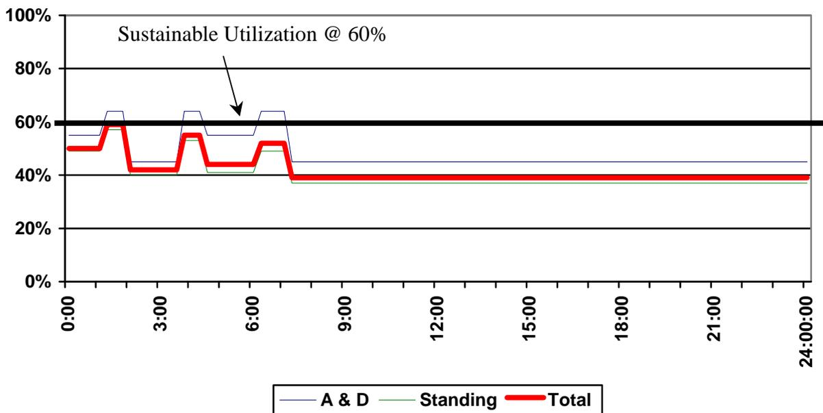
In the Base simulation, the daily utilization graph indicated that when a grain train was in Glen Yard, 40% to 50% of the total capacity of the yard was consumed. Sudden increases approaching 60% utilization were noted when transfers bringing empties back from the Waterfront arrived, but those spikes receded to more average levels when the shuttles left with loads destined for the elevators. Under these operating conditions, Glen Yard is not capacity constrained.
