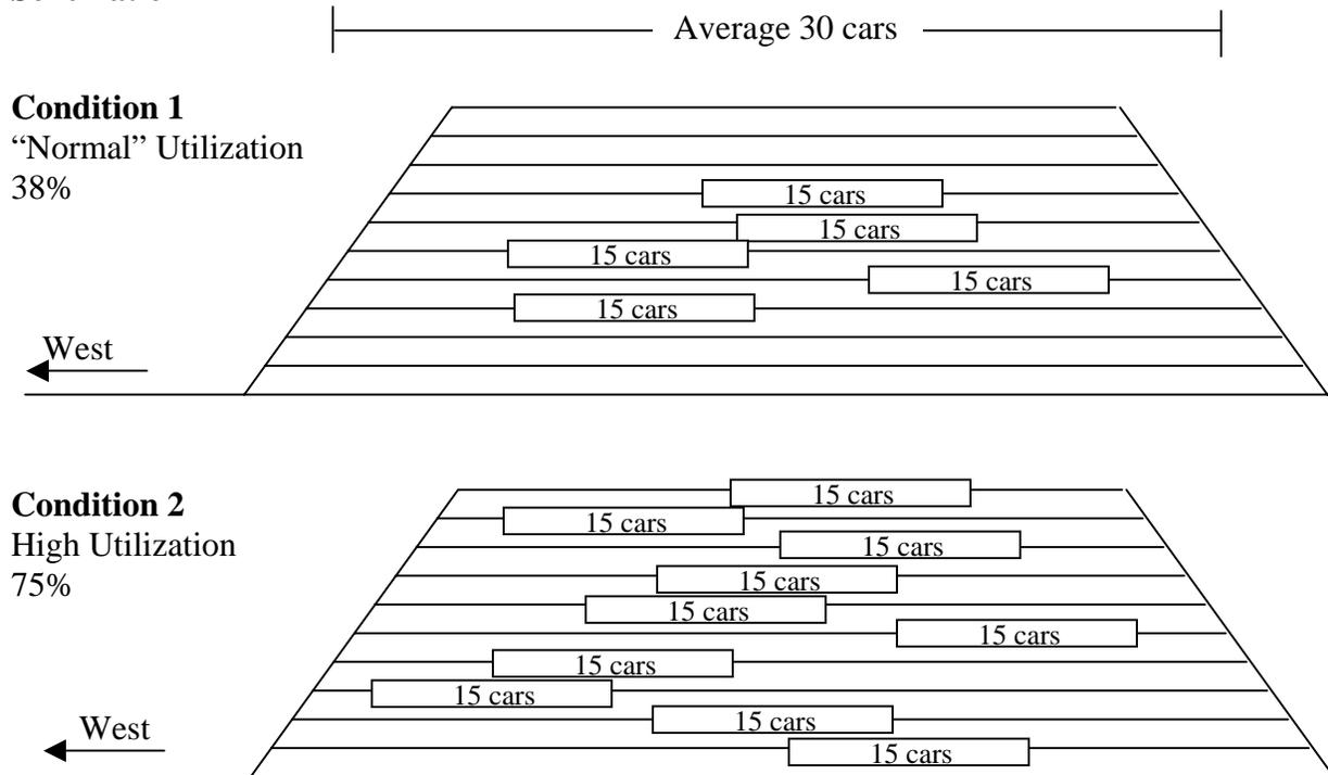
For this example, also assume the yard has a main line track running past it from east to west. If a 60-car westbound train needs to arrive into this yard in Condition 1 (normal operations), it
