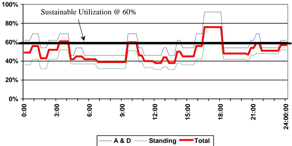
Even though the capacity consumed over the simulated day does not regularly exceed sustainable levels, the track usage chart for Main Yard (Exhibit 8) clearly shows that all tracks in the yard are used regularly throughout the day. During periods when a large transfer arrives (such as at 1600), up to 90% of tracks had cars on them for approximately two hours (A/D line in the graph). This is an indication that all available tracks were necessary for the operation to be accomplished.
