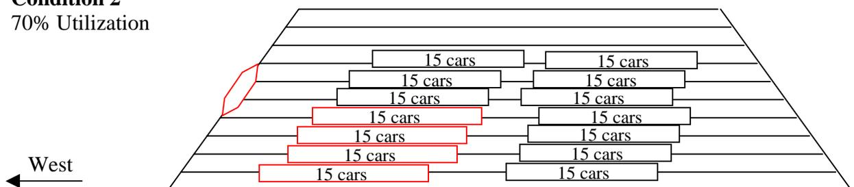
Once room is created, the switch engine can now couple to the cars that need to be switched, pull them west of the yard, and marshal them into the empty tracks. As mentioned previously, it is convenient that there are only three blocks necessary and there are three tracks available. If a fourth block was required, cars would have to be switched back into one of the tracks the cars were pulled from, leaving a portion of the track marshaled while the rest of the track was not switched.
