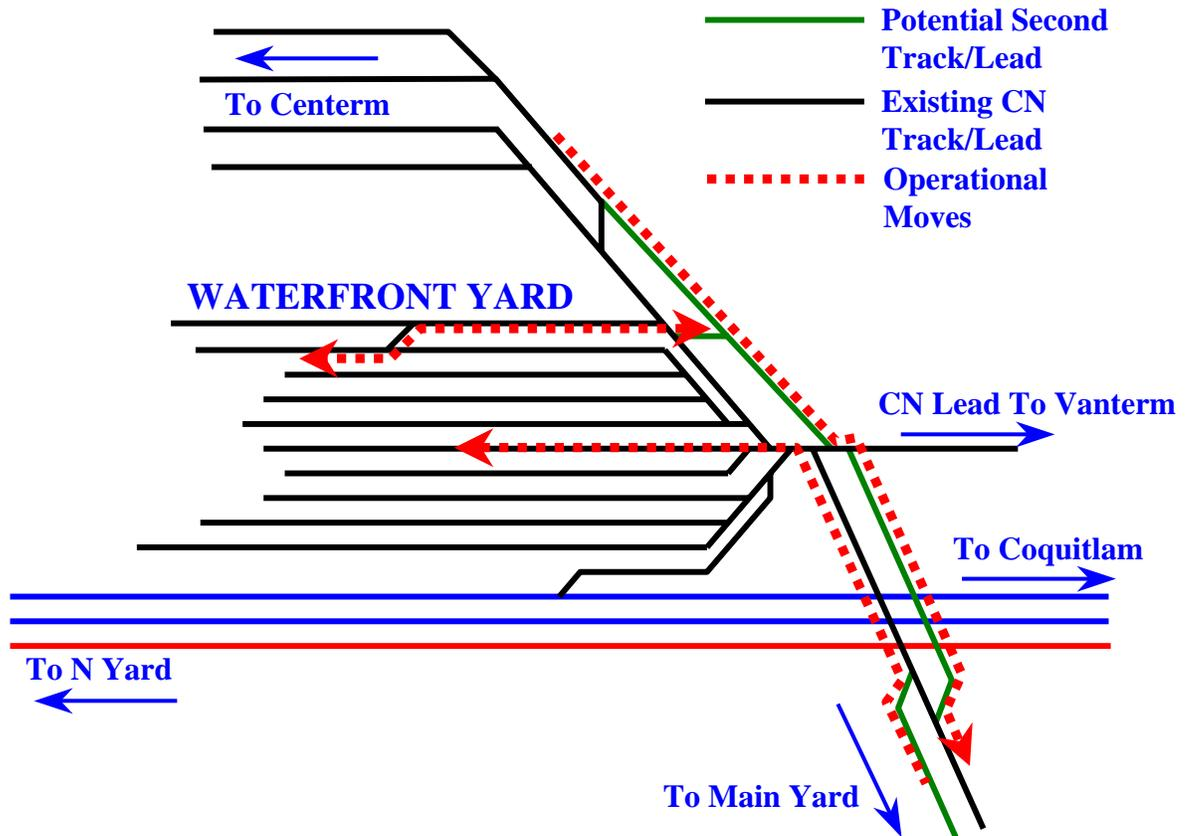
The configuration is designed to allow a move of CN traffic from Centerm to Main Yard to be made simultaneously with a move from Main Yard to Waterfront Yard. The configuration would also allow a pull or spot of CP Centerm traffic to/from N Yard to occur simultaneously with a move to/from Main Yard (see Appendix 3 for more details on the requirements for this type of move).
