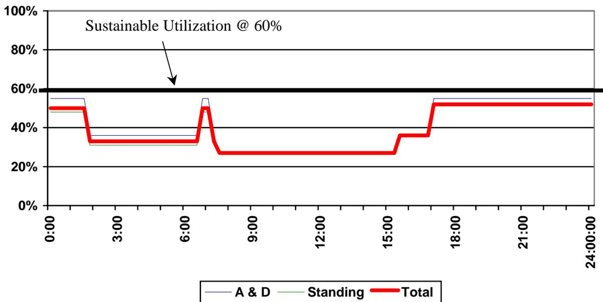
In the Future simulation, capacity consumption within the yard was again predicated on when loads arrived from Thornton (or Main Yard) and/or empties arrived from the waterfront. The utilization of the yard clearly indicated that not all available tracks were used, as the A/D percentage never exceeded 60%.
