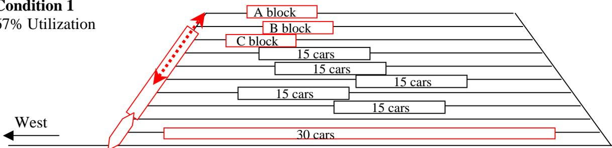
The yard would be configured as shown in Schematic 3 as the first track was switched. At the completion of switching one of the two tracks, the total capacity utilization percentage would be 67% (A/D = 90%, standing = 45%). When both tracks have been switched, the utilization percentage reduces to 62% (A/D = 80%, standing = 45%). As this example demonstrates, a yard
