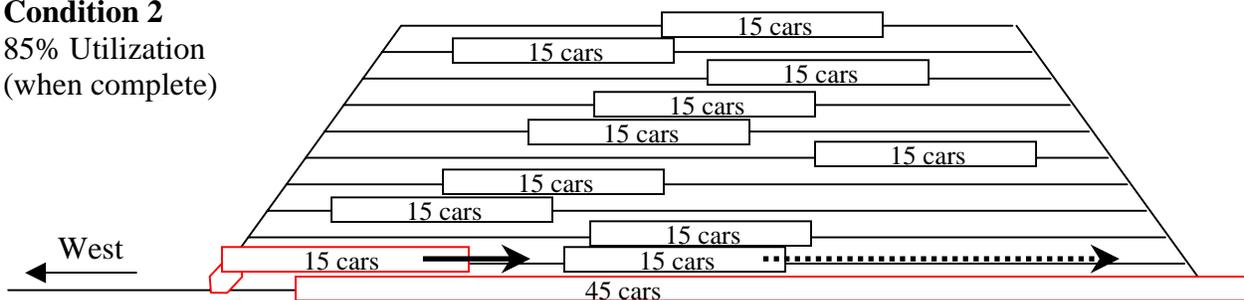
An arrival process of this nature would likely take 1.5 to 2 hours because each cut of cars being moved into the yard tracks has to be ridden by the train crew employee to make sure they don't collide with the cars already in the tracks. Additionally, if the cars in the track are not sitting at the east-end of the track, the employee would have to couple the cars on the train to the cars in
