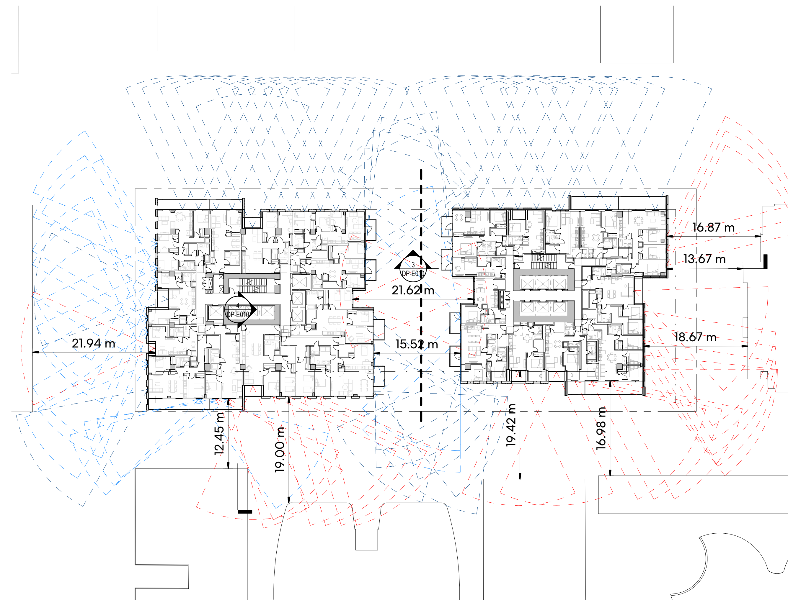
1 Podium Horizontal Angle of Daylight 1:400
