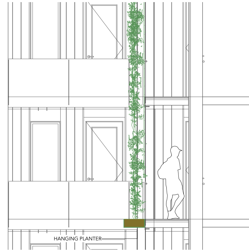
3 SECTION D-D VERTICAL CABLE TRELLIS Scale: 1:30
