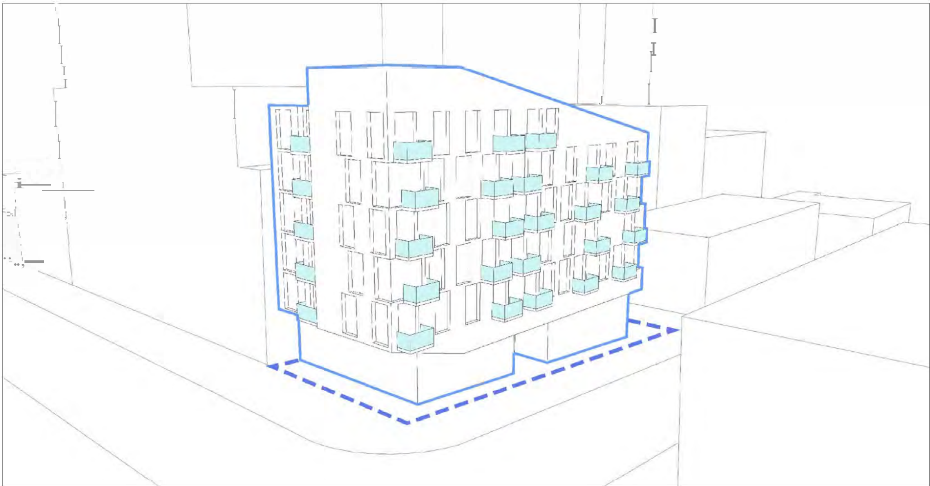
PHASE 7: Each suite has access to outdoor space via a private balcony. The structural steel balconies are 'hung' off the facade to further improve the thermal performance of the building envelope.
