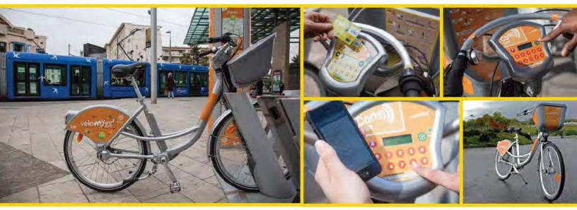
Smoove bicycles are safe, reliable, and durable for all weather conditions. The enclosed drive train and fenders protect the bicycle from damage due to inclement weather. The bicycles are comfortable and adjustable to accommodate all riders without tools, and feature flat pedals, puncture-resistant tires, and a kickstand for convenience. All Smoove bicycles can be equipped with GPS.
