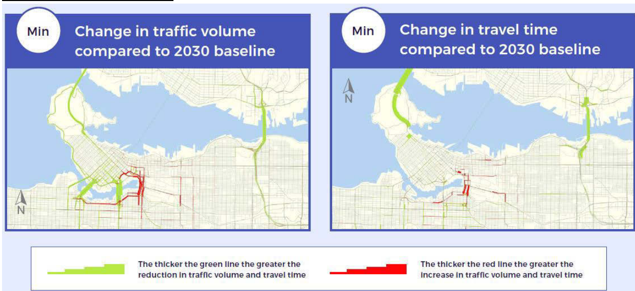
Figure 7: Map of traffic volumes and modelling of regional congestion point charges on the False Creek Bridges .
