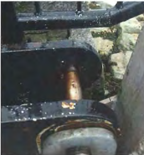
Westerly Roller bottoming out causing wear on frame and dragging ramp with float motion for excessive motion at top of ramp.
