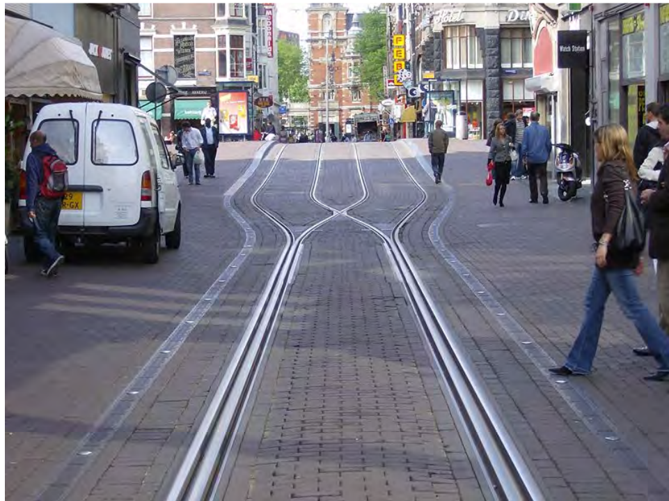
Figure 3-16 Interlaced track in Leidsestraat in Amsterdam
