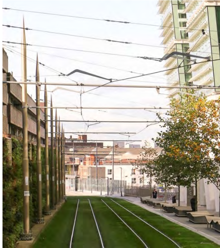
Figure 4-15 Decorative poles with cantilever supports in Birmingham
