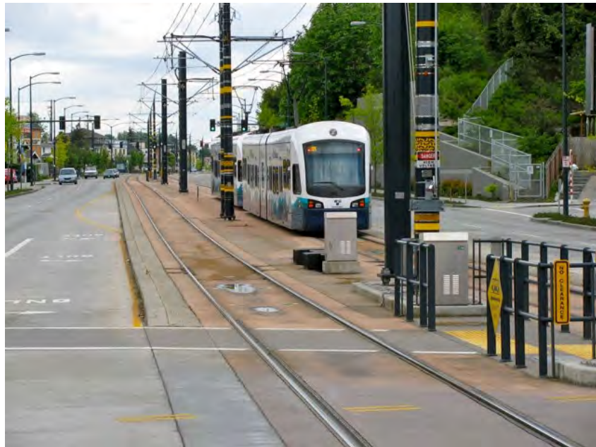
Figure 3-12 In-street Segregated Trackway, Seattle
