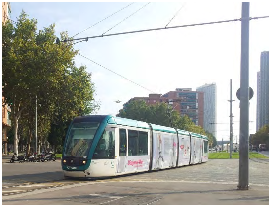
Figure 4-16 Single Wire OCS in Barcelona
