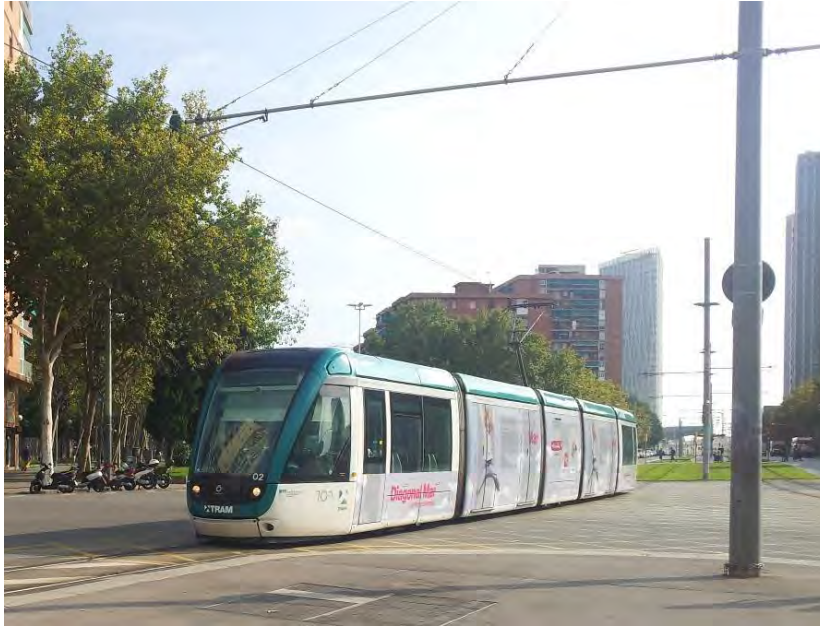
Figure 6-4 Single wire OCS in Barcelona
