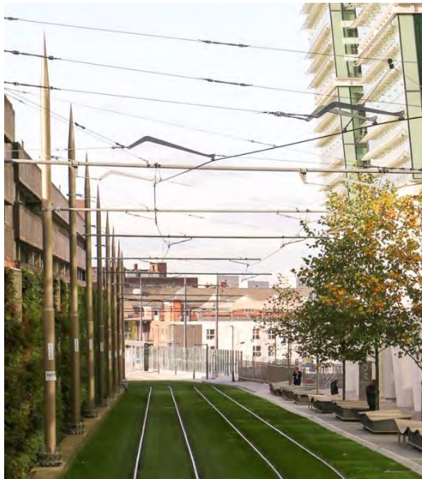
Figure 6-3 Decorative poles with cantilever supports in Birmingham
