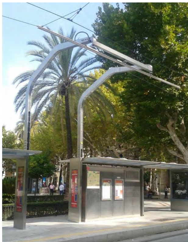
Figure 6-7 Charging point at a stop – Seville, Spain
