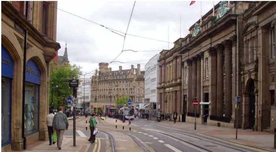
Figure 6-6 Span OCS wires affixed to buildings, Sheffield, UK
