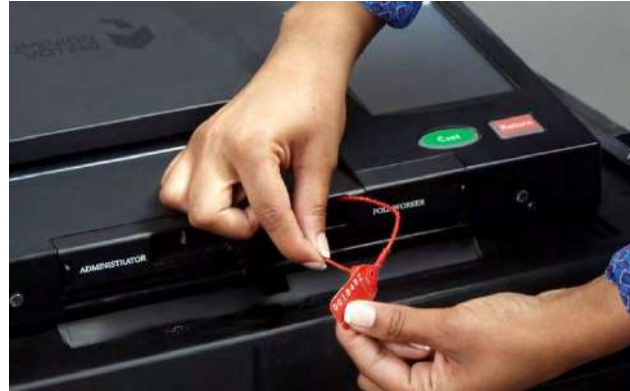
Memory Card Compartments sealed for security
