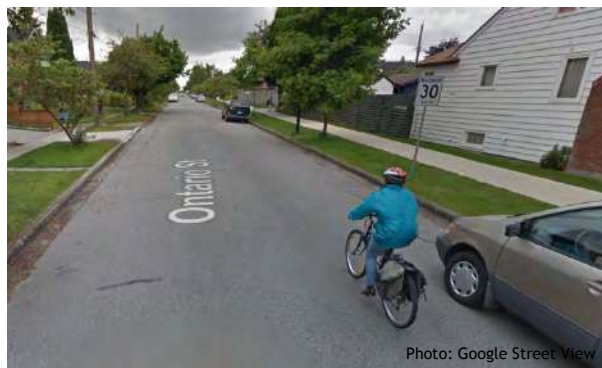
Figure 7: Ontario St near 27 th , 8.2m (27ft) curb to curb. In this example, there is low to moderate parking utilization on a narrow bikeway. This creates numerous pockets where a cyclist can comfortably pass an oncoming vehicle. For these situations, engineering judgement on a case by case basis can be used to determine suitability as AAA.
