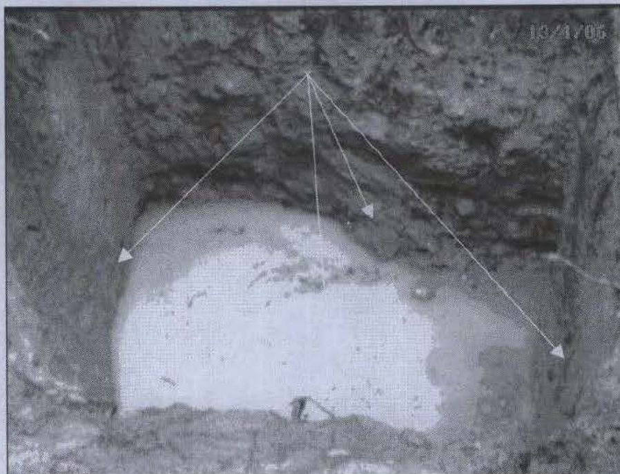
Sampling locations (note oil still floating on the groundwater surface)
