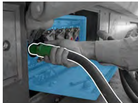
3. Working in sequence LEFT to RIGHT , lift each coloured flap in turn and install the matching coloured cable before moving to the next cable until all 5 are connected:
