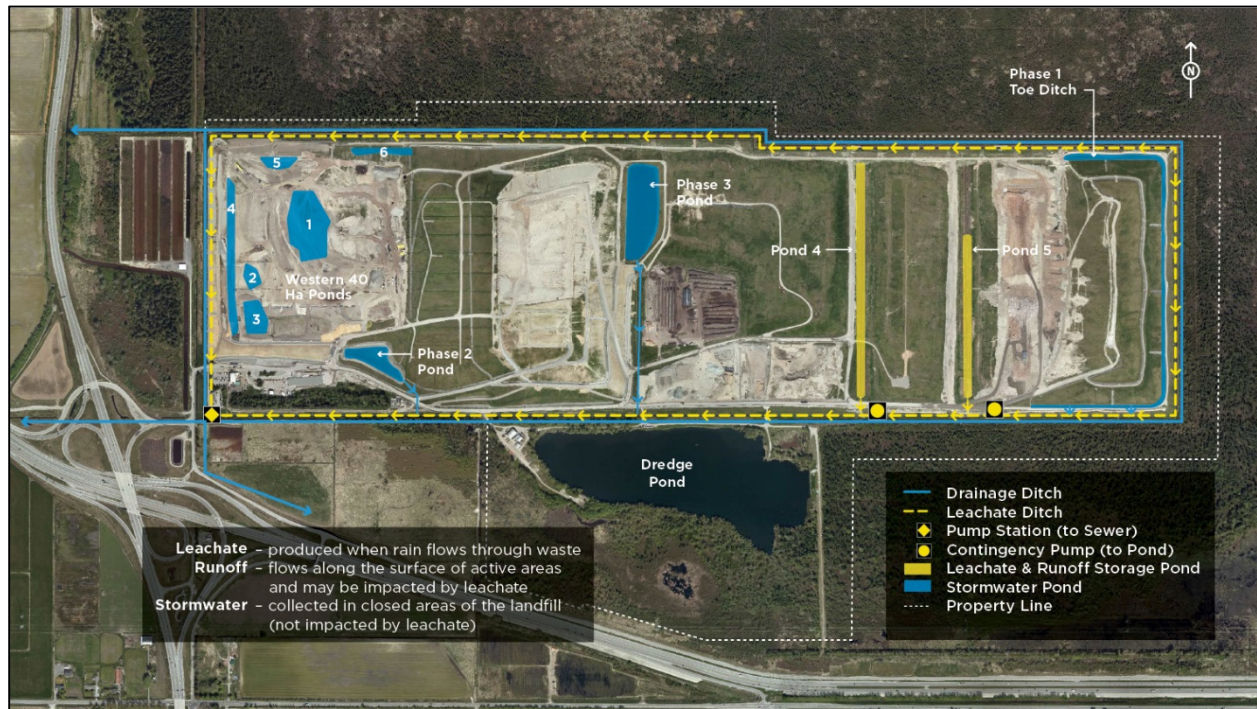
Figure 5: Leachate, Surface Runoff and Stormwater Management
