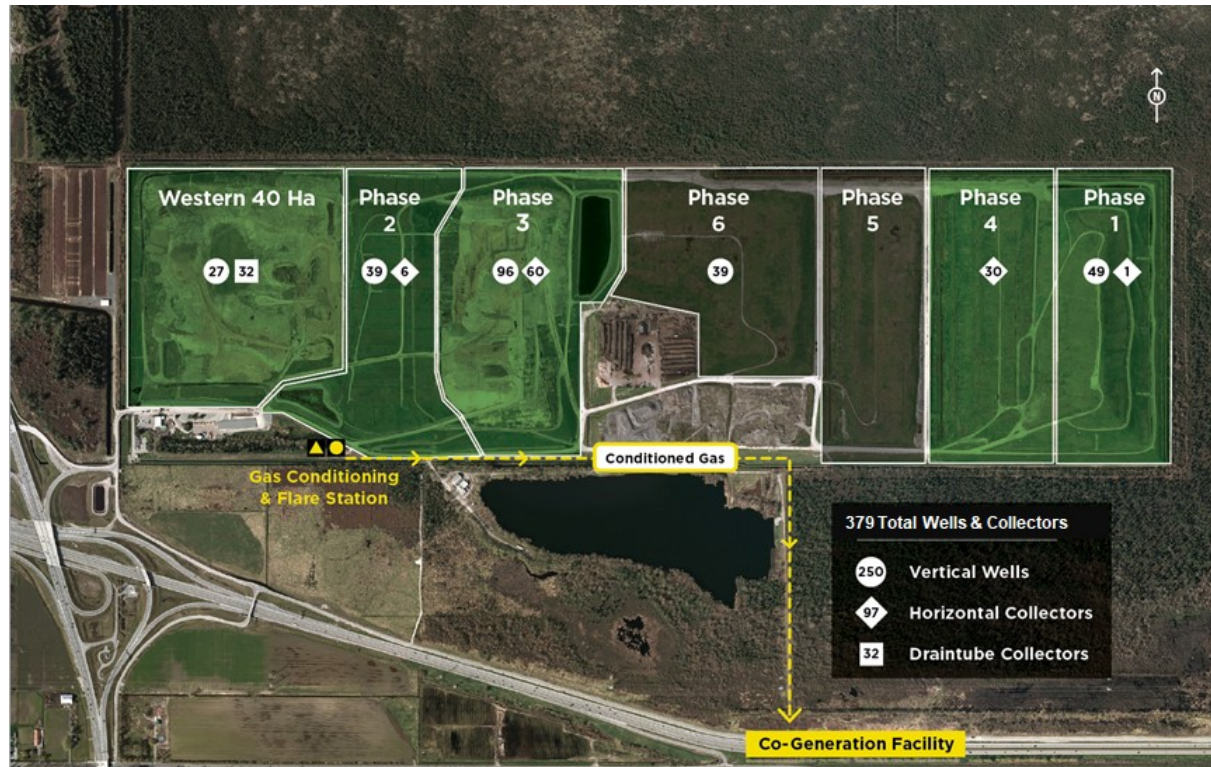
Figure 9: 2019 Landfill Gas Collection System
