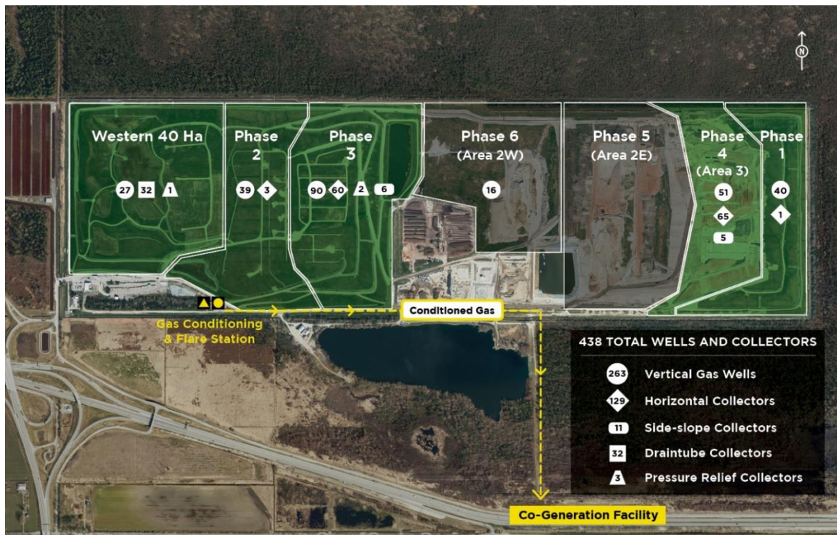
Figure 9: 2021 Landfill Gas Collection System
