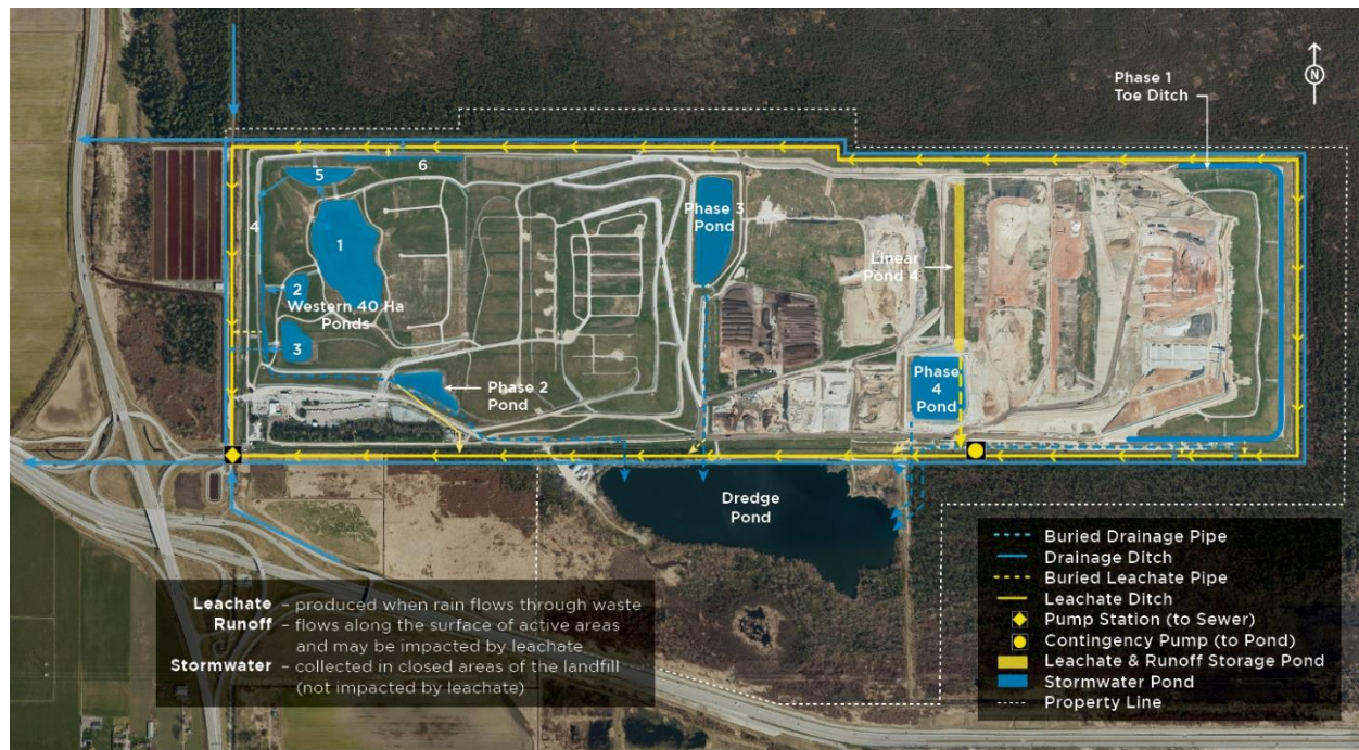
Figure 5: Leachate, Surface Runoff and Stormwater Management
