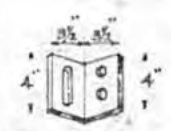
ISOMETRIC VIEW OF ANGLE CONNECTION SHOWING SLOTTED HOLE
