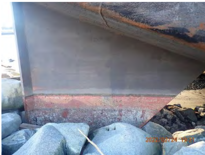
Photo 24 East Groyne - starboard rudder of barge has dug into groyne, southward view.
