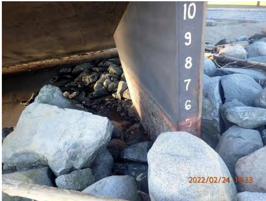
Photo 25 East Groyne - starboard rudder of barge has dug into groyne with approximately 1 m gap south of rudder, westward view.
