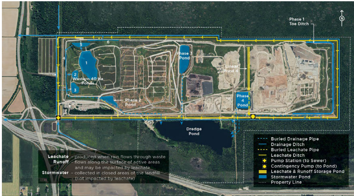
Figure 4: Leachate, Surface Runoff and Stormwater Management
