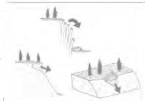
Figure 5: Rock slope failure mechanisms
