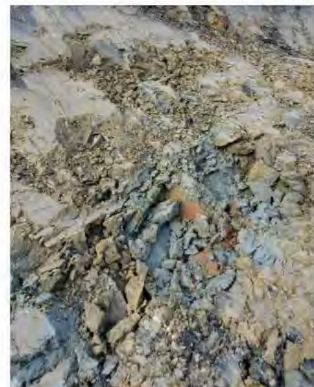
Photo 16: Oxidized sub-vertical discontinuity in Vashon Deposits
