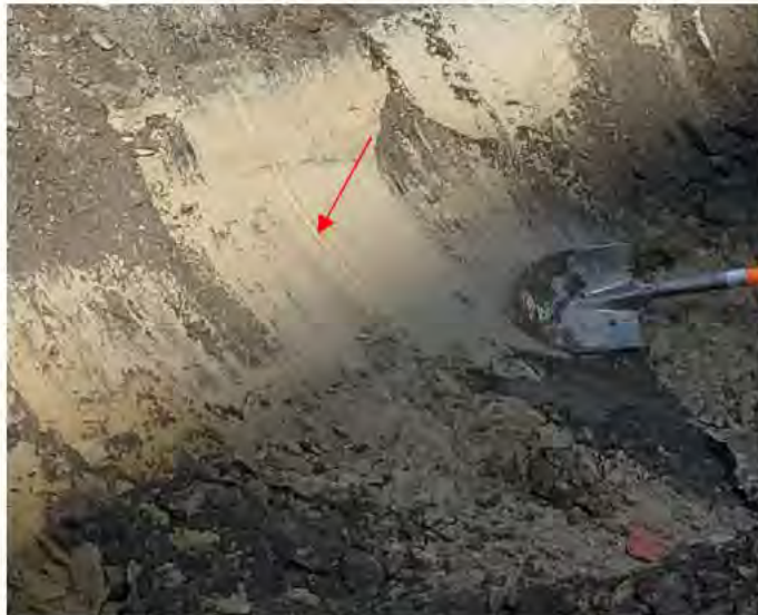
Photo 15: Vertical discontinuities in Capilano Deposits
