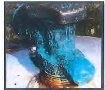
**Signs to Look For:** A blue-green stain on any brass portion of a service valve indicates it may have been in contact with anhydrous ammonia. The pungent odor of ammonia (a window cleaner smell) is also an indicator.
