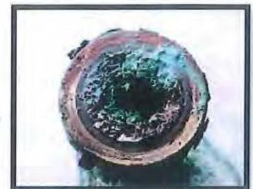
**Recommended Action:** If you suspect a propane cylinder contains/has contained anhydrous ammonia; has been tampered with; or overly exposed to the elements and has degraded in integrity: 1) Do not touch; 2) Secure it so others don't touch (eg. flagging tape); 3) Notify your supervisor; and 4) call Environmental Emergency Response Team at 604-450-3493 to dispose.
