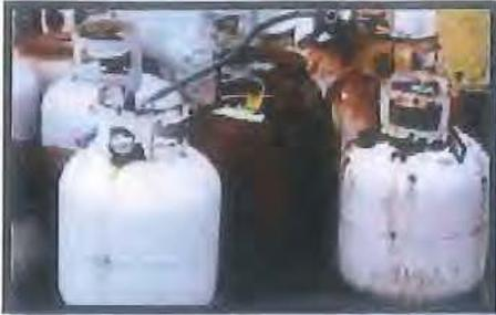
**2** - Corrosion on the body or valve stems can lead to failure or rupture at the weak point, creating shrapnel-like projectiles with a sudden pressure release.
