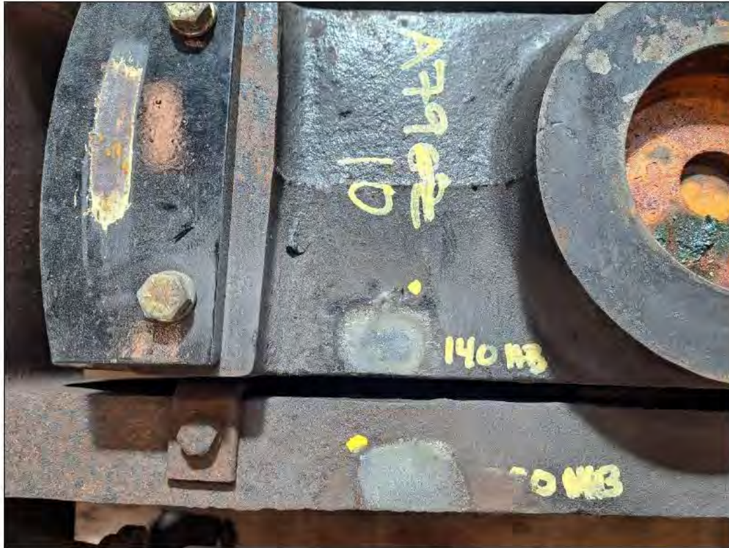
Figure 14 Areas tested for microstructure and hardness.
