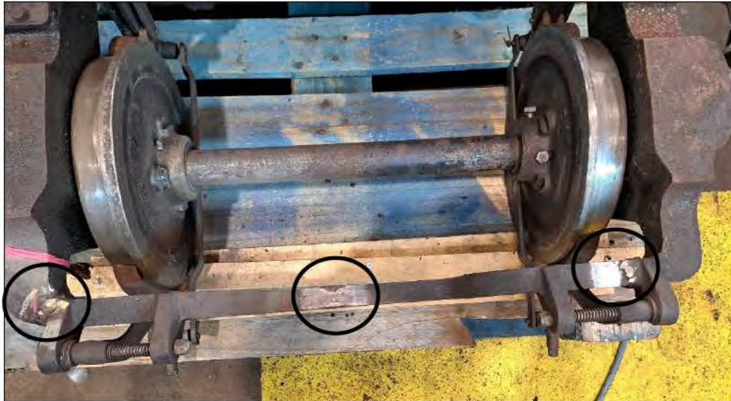
Figure 12 Repairs found that used copper filler.
