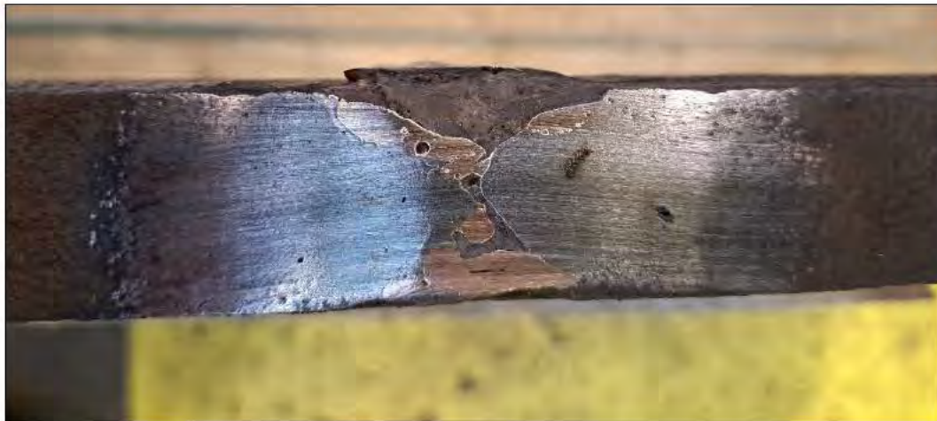
Figure 13 Repairs found that used copper filler
