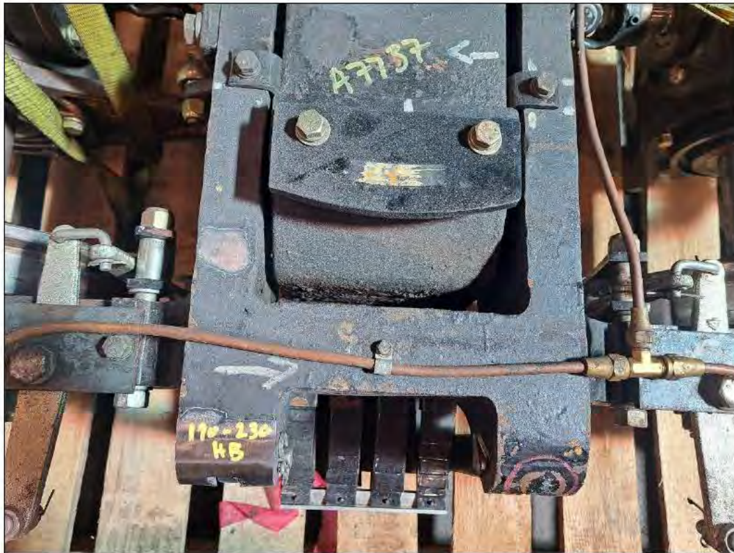
Figure 15 Area polished to identify any weld repairs – none found.
