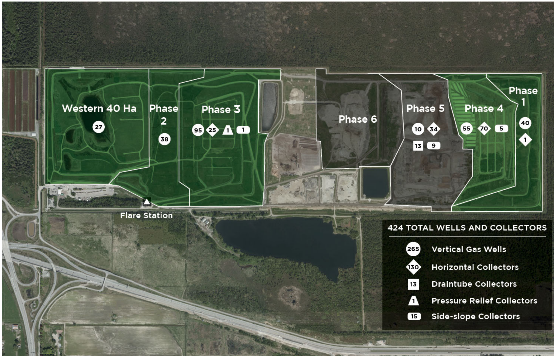
Figure 7: 2023 Landfill Gas Collection System
