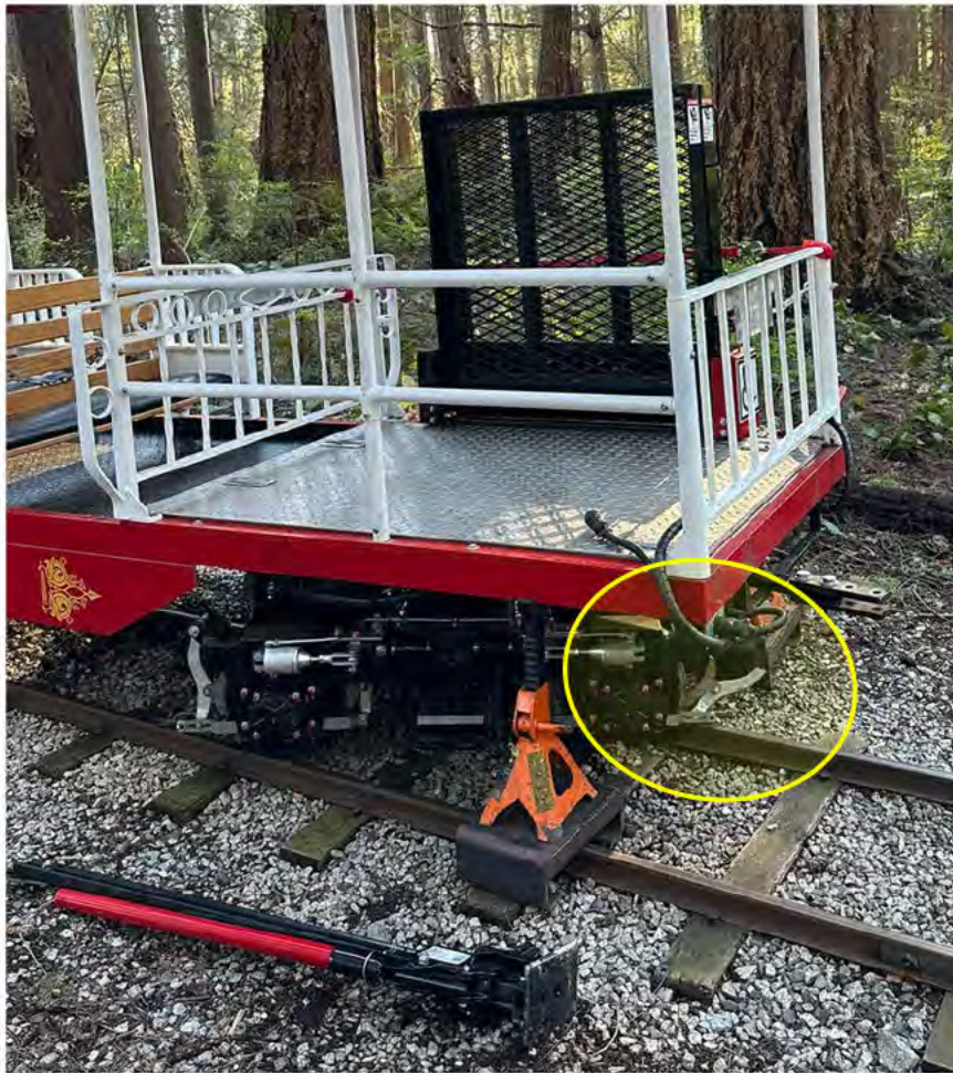
Figure 2 - Derailed Carriage (damaged brake linkage highlighted)
