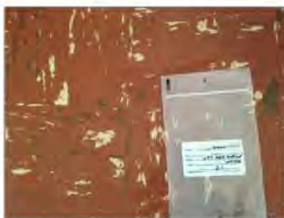
Asbestos-containing vinyl floor tiles.
