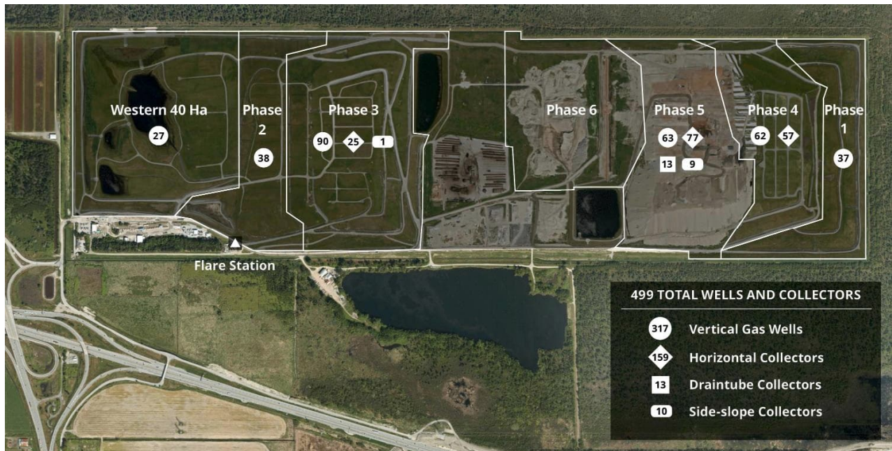
Figure 7: 2025 Landfill Gas Collection System
