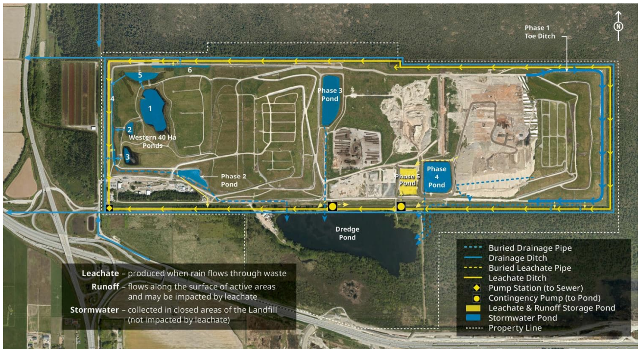
Figure 5: Leachate, Surface Runoff and Stormwater Management
