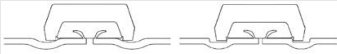
Figure A-2.2.10.4.(1) Insufficient Key Engagement of Fitting in Roll Grooved Connection
