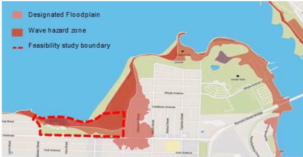
Figure 3 –City of Vancouver 2014 Open Data Portal showing existing floodplain and wave hazard zone
