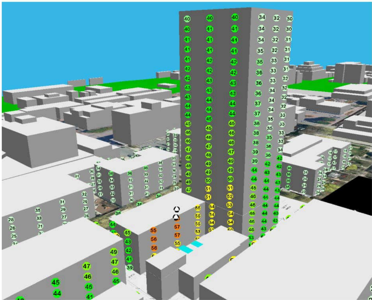
Figure 4: Predicted Future Noise Levels – Mechanical Equipment Only
