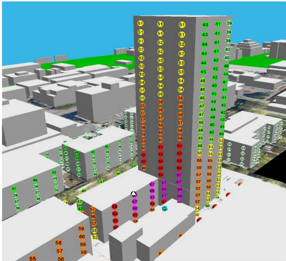
Figure 5: Predicted Future Noise Levels – Generator Only
