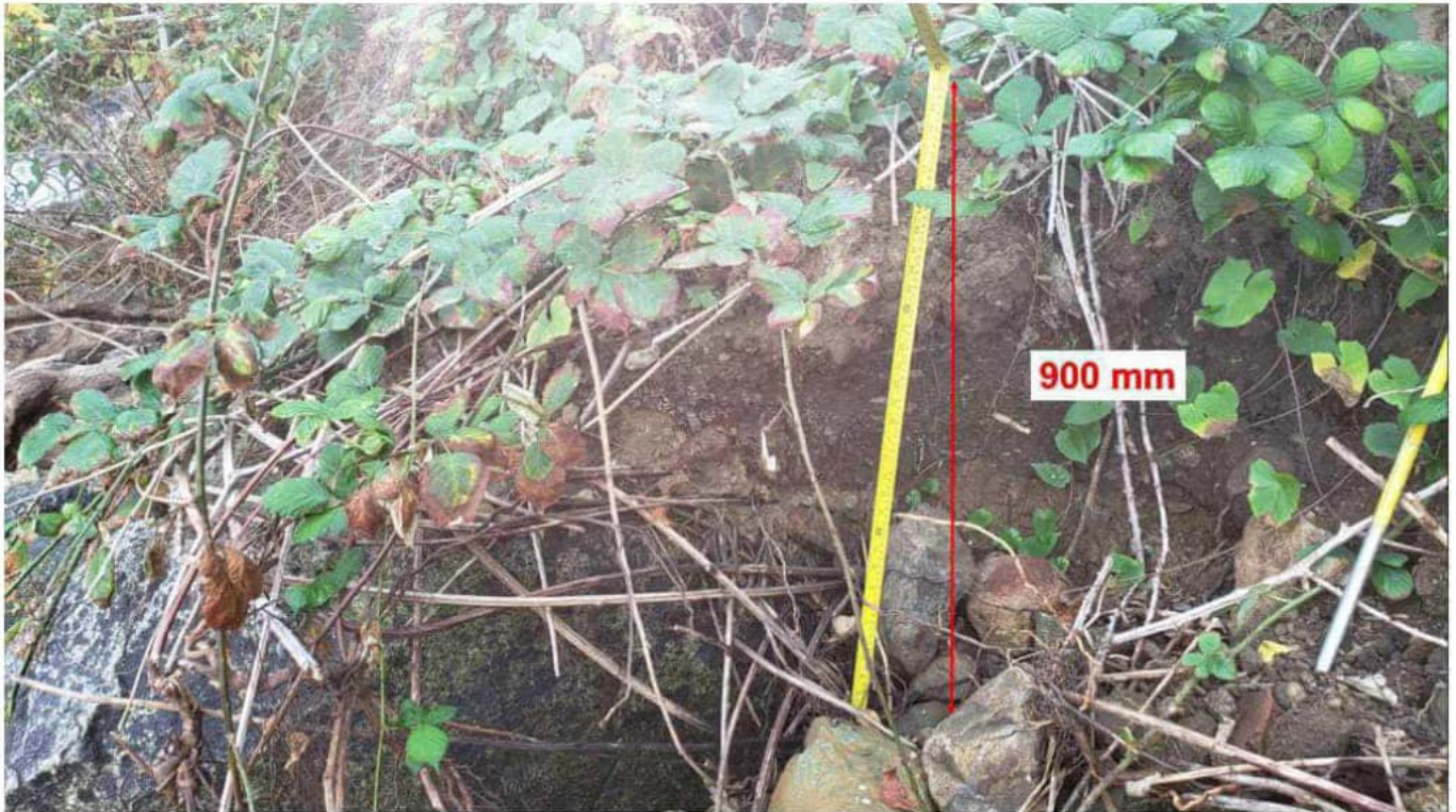
Photograph 3: 900 millimetre thick deposit of colluvium/landslide debris at bottom of North Slope
