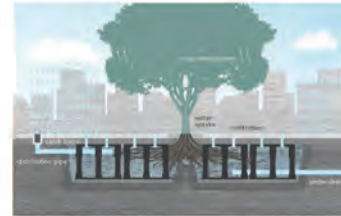
Silva cell under hard paving
