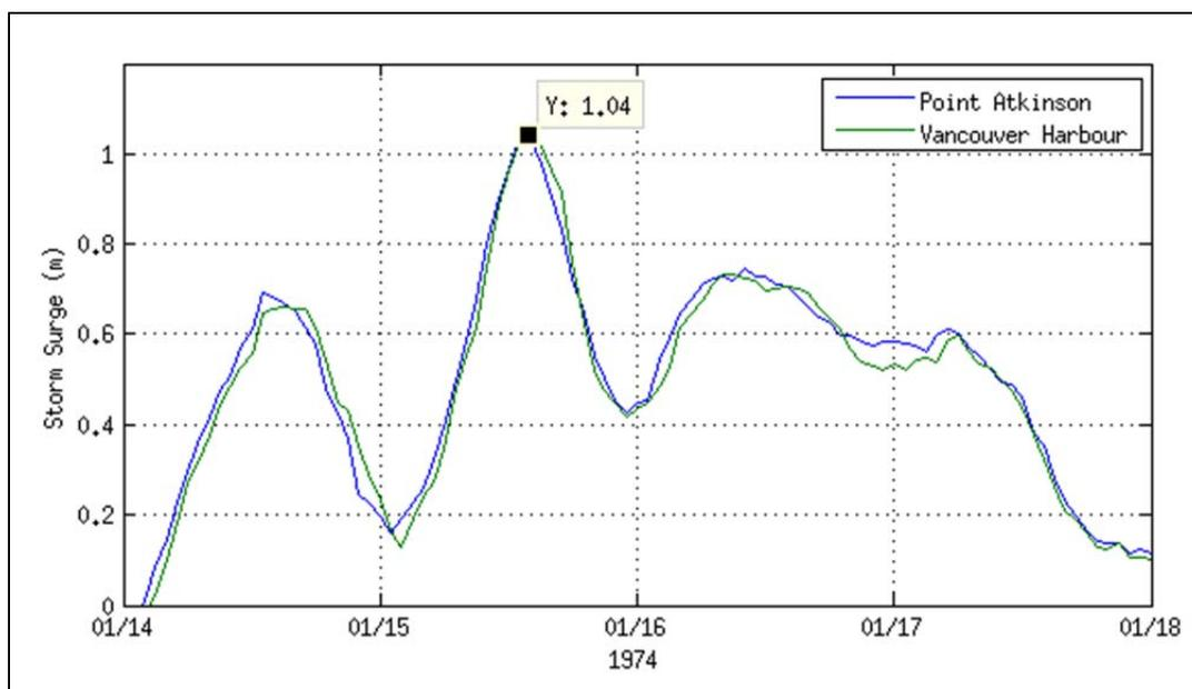
**Figure 8. Tidal residual calculated at Point Atkinson and Vancouver Harbour.**
