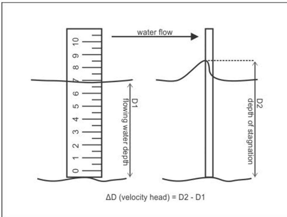
Figure 20. Using a metre-stick to measure velocity head.
