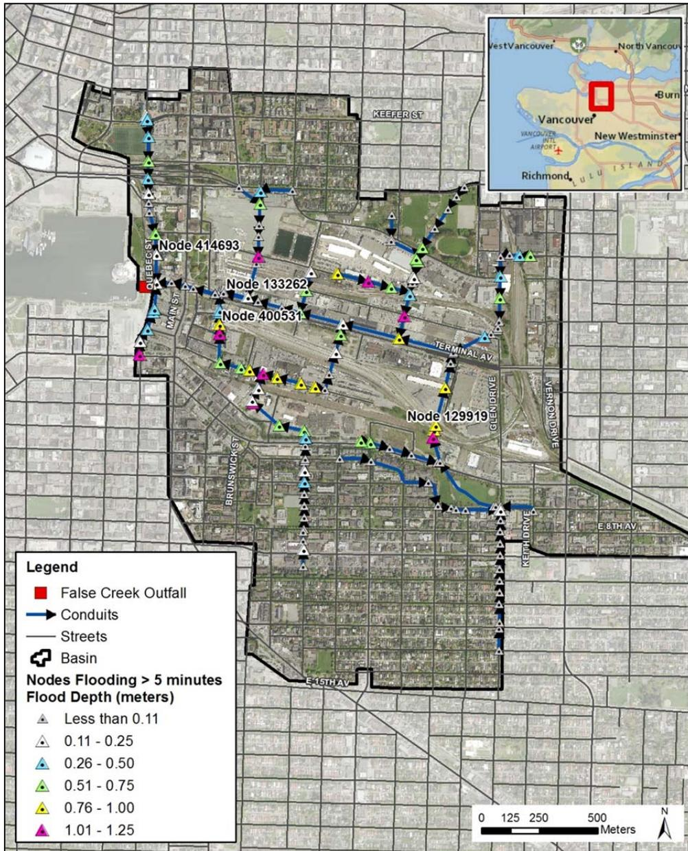
Figure 36. Simulated flooding depths for Scenario 3 with a 25-year design storm.
