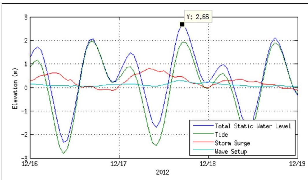
**Figure 12. Hindcast components of water level for the December 2012 King Tide event.**
