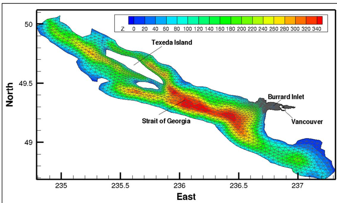
**Figure 10. Wave model grid and colour contours of bathymetry (m).**
