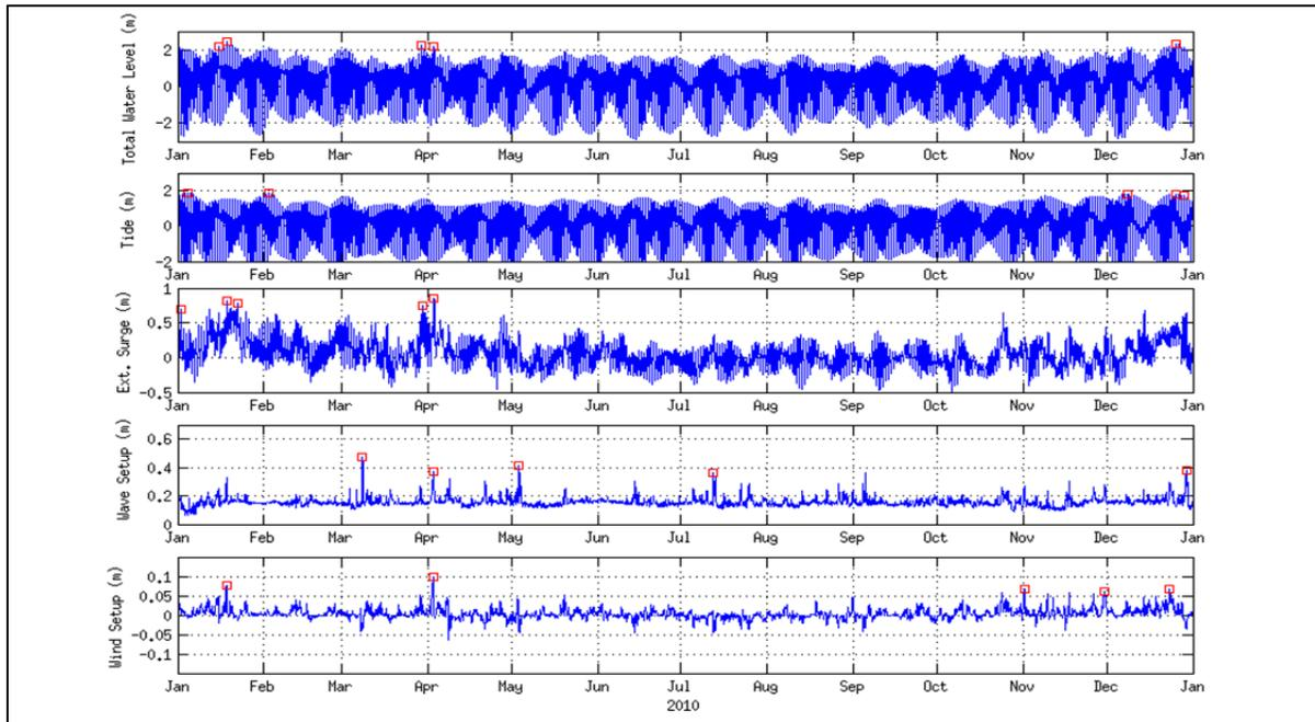
**Figure 5. Time-series of each of the components of sea level at False Creek for the year 2012. Red boxes isolate the five highest values in the time-series.**
