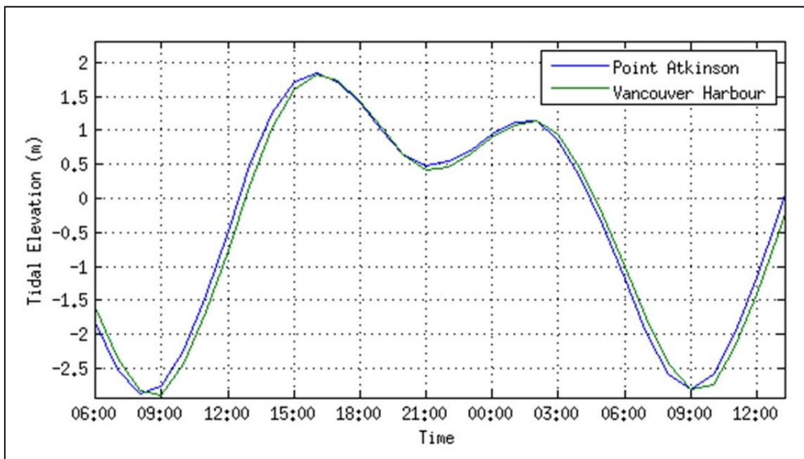
**Figure 7. Tidal elevation (m GD) at Point Atkinson and Vancouver Harbour during a spring tide.**
