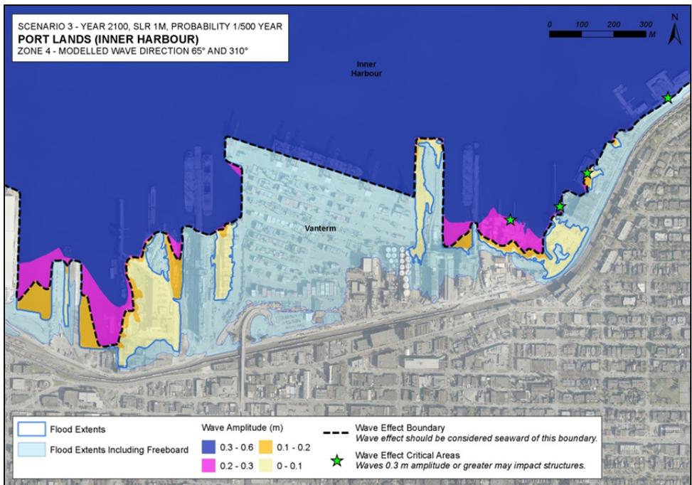
Figure 28. Scenario 3 modelled wave effects – detail of Port Lands (Inner Harbour).
