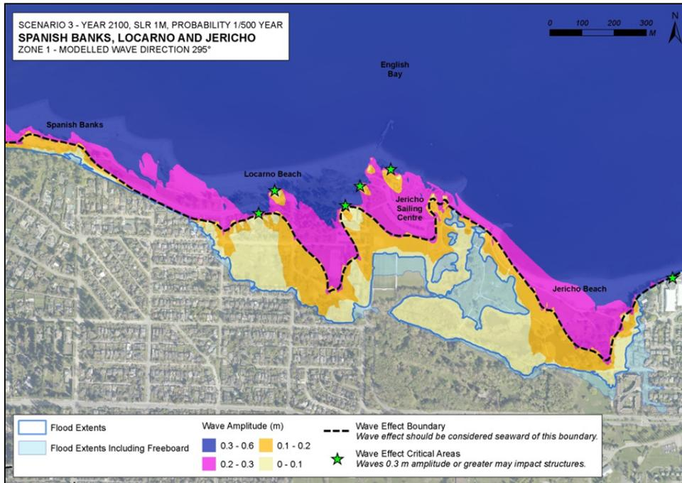
Figure 22. Scenario 3 modelled wave effects – detail of Spanish Banks, Locarno and Jericho.
