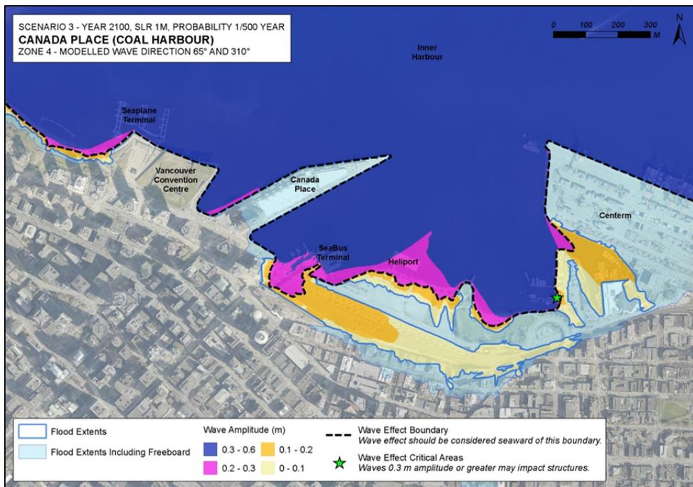
Figure 27. Scenario 3 modelled wave effects – detail of Canada Place (Coal Harbour).
