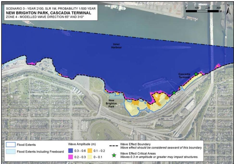
Figure 29. Scenario 3 modelled wave effects – detail of New Brighton Park, Cascadia Terminal.
