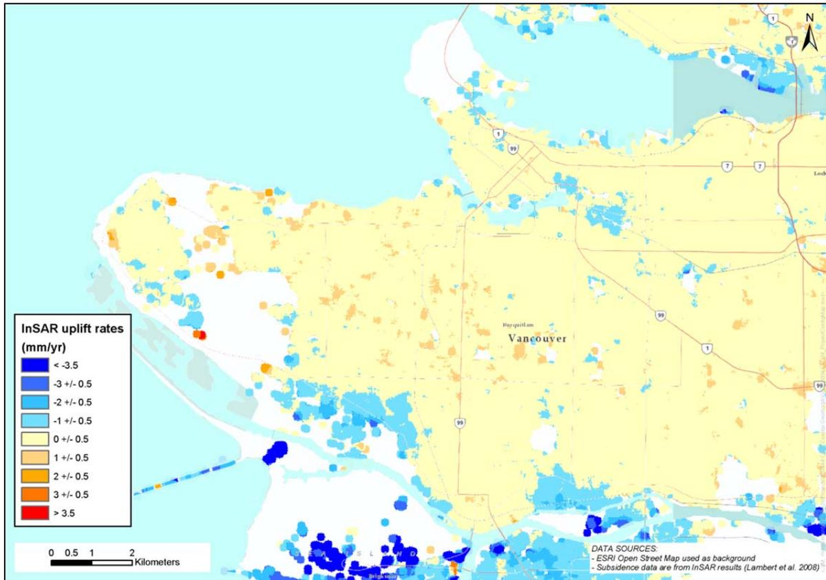
**Figure 4.** Map showing the rates of ground elevation change for the City of Vancouver (various sources - from Hill et al., 2013). Positive values indicate uplift and negative values indicate subsidence.
