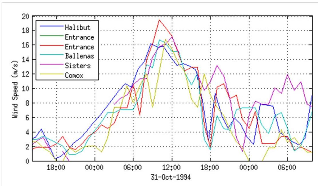
**Figure 9. Wind speeds measured at various stations on October 21, 1994. Wind speeds have been scaled to 10 m height and 1 hour averaging duration.**
