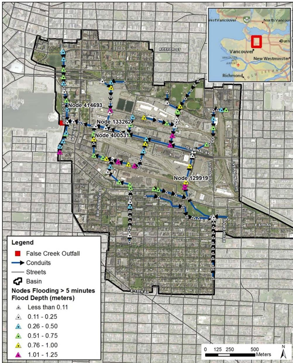
**Figure 37. Simulated flooding depths for Scenario 4 with a 25-year design storm.**
