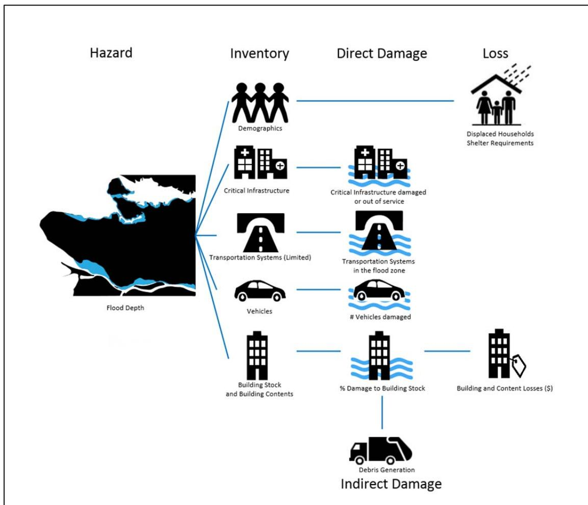
**Figure 40. Hazus modelling structure for City of Vancouver.**
