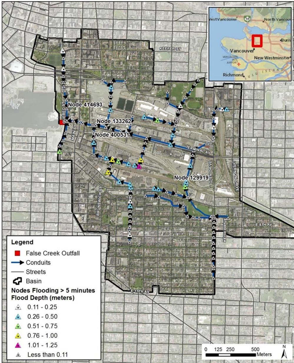
**Figure 34.** Simulated flooding depths for Scenario 1 with a 25-year design storm.
