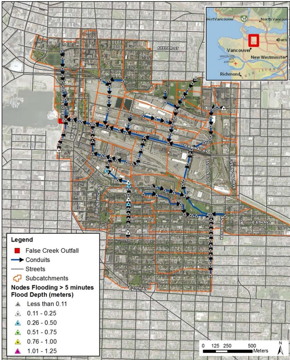
**Figure 33. Simulated flooding depths for a free outfall condition with a 25-year design storm.**
