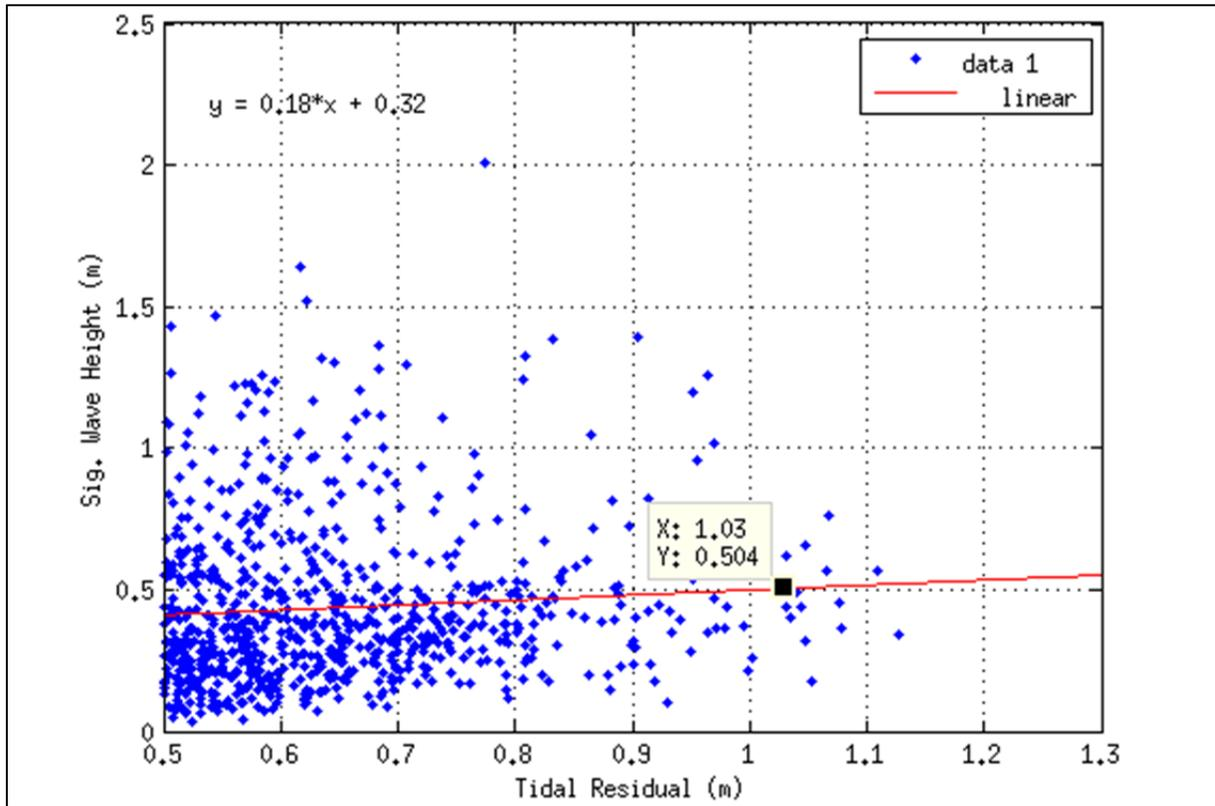
Figure 14. Hind-cast significant wave height during large tidal residual events.
