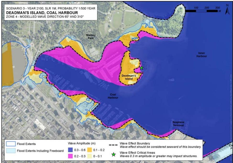
Figure 26. Scenario 3 modelled wave effects – detail of Deadman’s Island, Coal Harbour.
