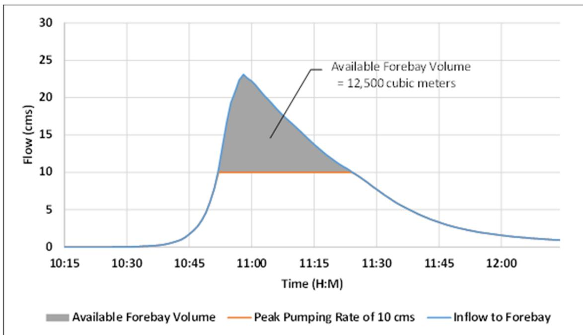
**Figure 39.** Hydrograph showing inflows to a pump station located at Quebec St. and Terminal Ave., forebay volume needed with a peak pumping rate of 10 m<sup>3</sup>/s is shaded grey.
