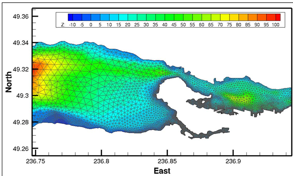
**Figure 11.** Wave model grid and colour contours of bathymetry, close up of Burrard Inlet.
