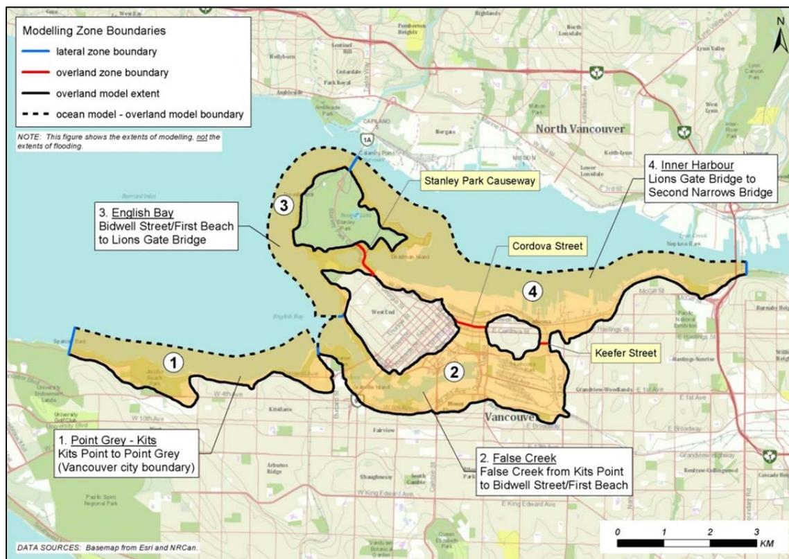
**Figure 15. Flood modelling zones in Burrard Inlet.**
