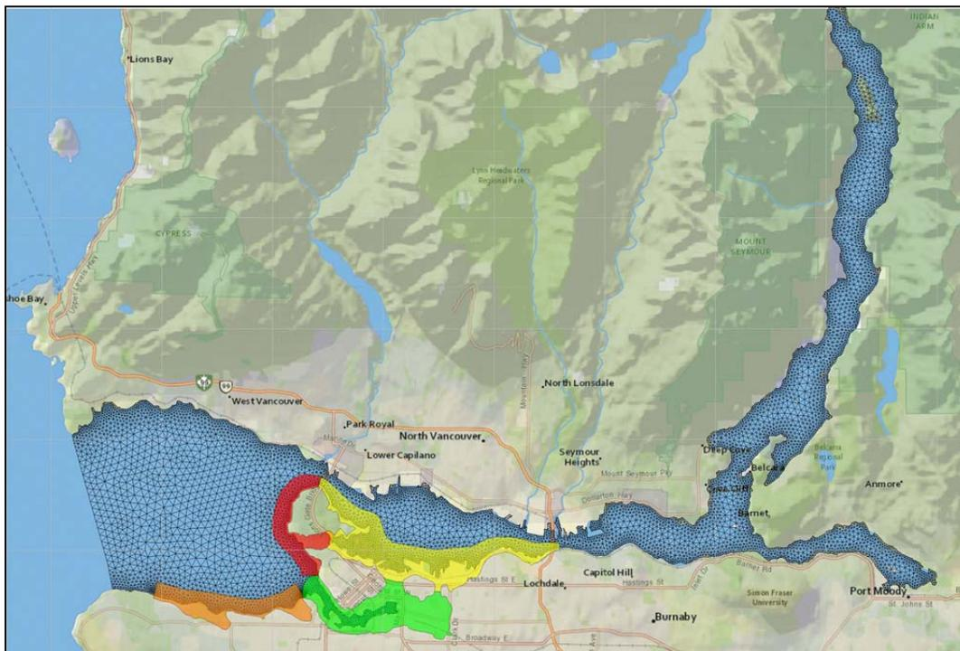
**Figure 16. Overland model extents with detailed sub-mesh areas for each zone shown in different colours (Zone 1 = orange, Zone 2 = green, Zone 3 = red, Zone 4 = yellow).**
