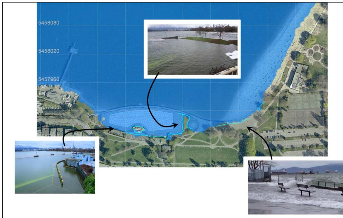
**Figure 19.** Comparison of observed and simulated flood extents at Kitsilano Pool and Beach for December 17, 2012.
