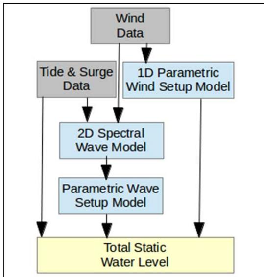
**Figure 6. Schematic of coastal hind-cast approach.**
