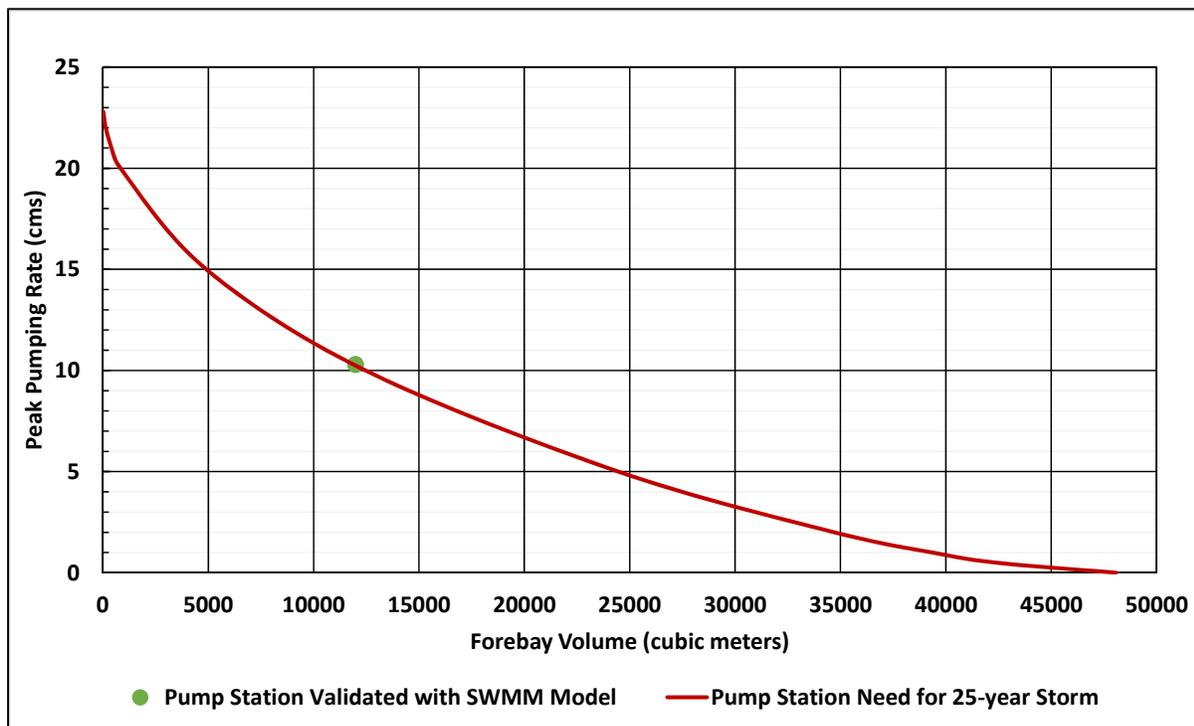
**Figure 38. Required forebay volumes and peak pumping rates for 25-year storm in the False Creek basin.**
