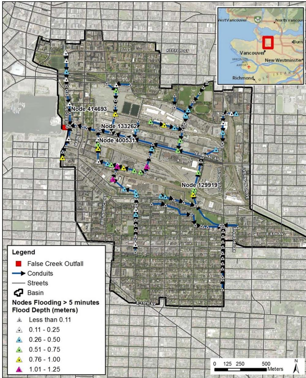
Figure 35. Simulated flooding depths for Scenario 2 with a 25-year design storm.
