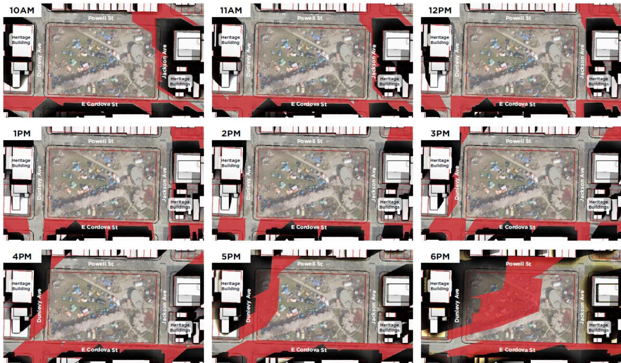
Figure 2: Openheimer Park Solar Study - Spring Equinox (March 21) from 10am-6pm; based on proposed built form envelope with new shadows in red (for illustrative purposes only).
