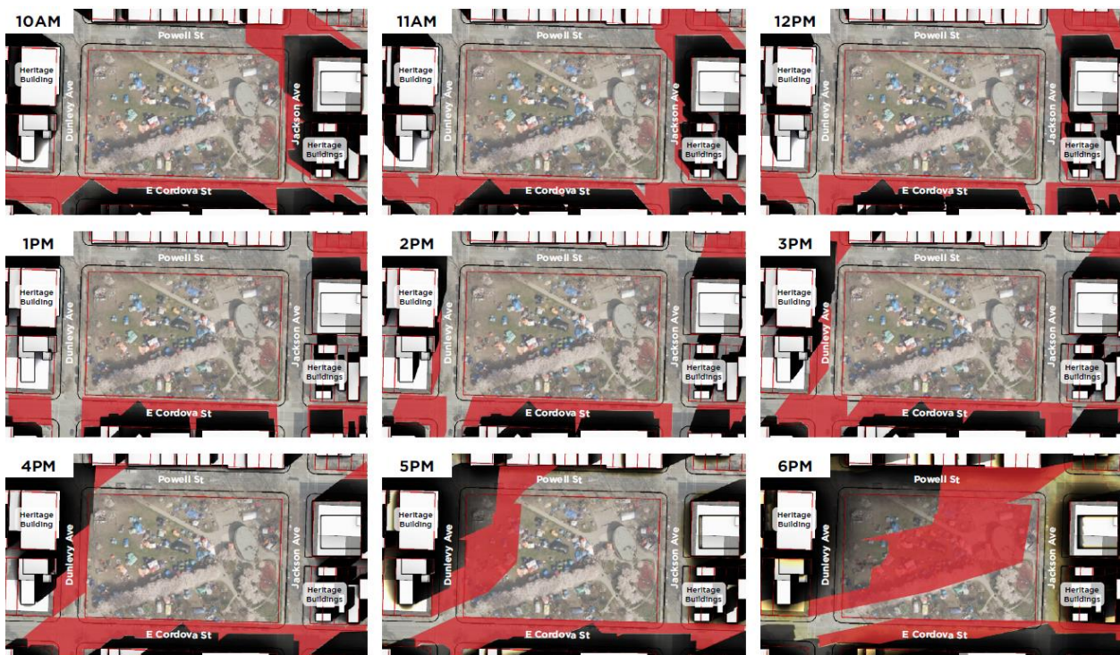
Figure 3: Openheimer Park Solar Study- Fall Equinox (September 21) from 10am-6pm; based on proposed built form envelope with new shadows in red (for illustrative purposes only).
