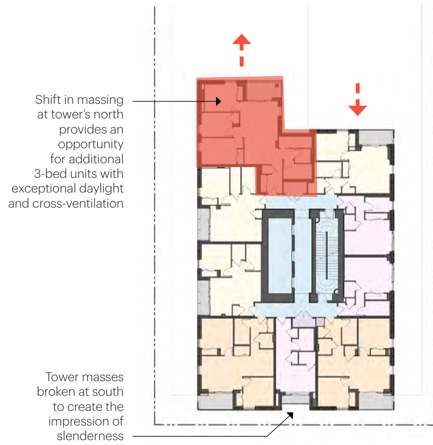
Tower floor plate shape
