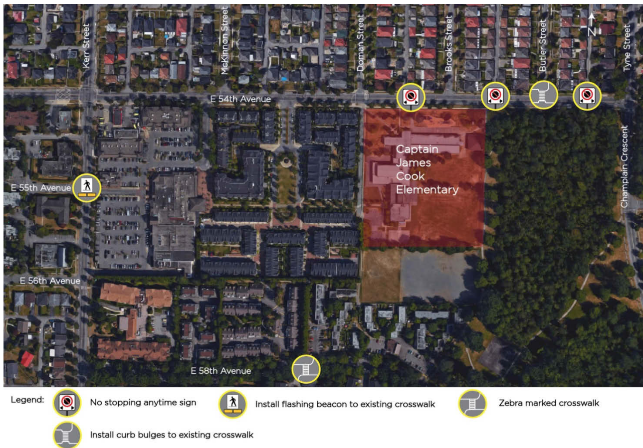
Figure ES.1 - Proposed infrastructure upgrades
