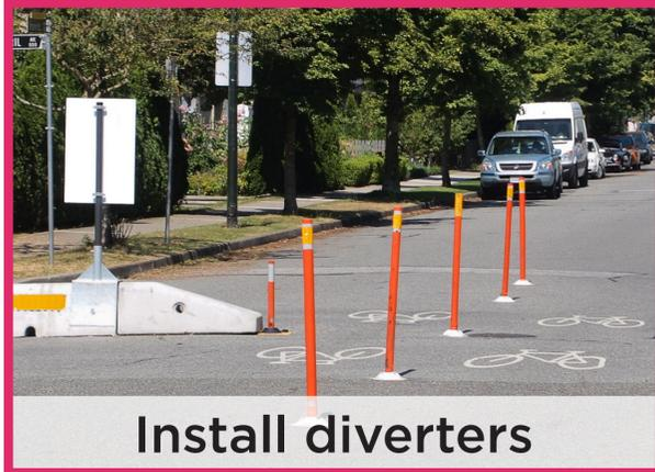
Barriers restrict the types of turns vehicles can make, while still allowing people walking and cycling to travel through the barrier. This can reduce vehicle short-cutting as an indirect route is less desirable.
