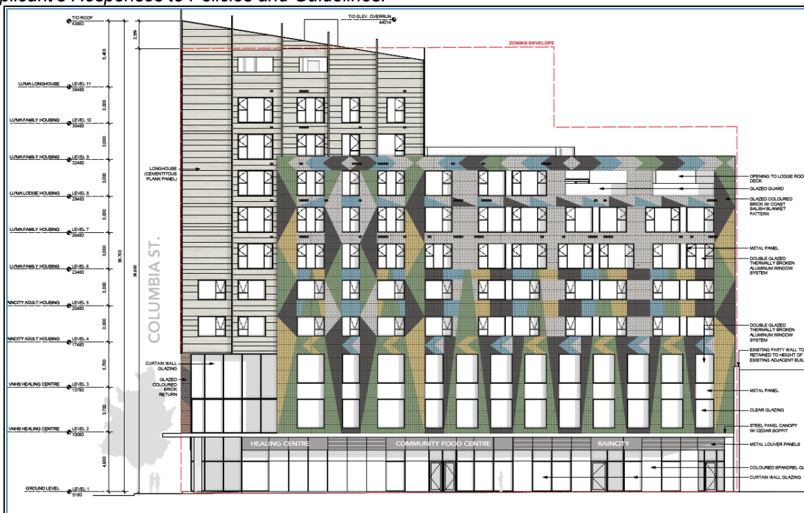
Fig 1: Hastings Elevation Red dash line shows the intended height/massing per the DEOP Plan.
