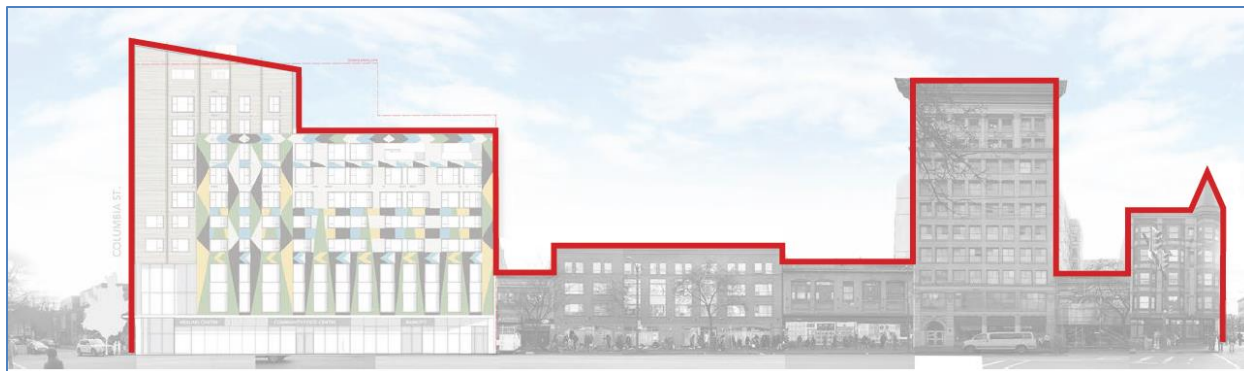
Fig 2: Block - Hastings Elevation Red line indicates the saw-tooth roof profile expressed at a block-scale.
