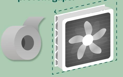
Find the directional arrow on the side of the filter. Place arrowfacing the back of the fan.
