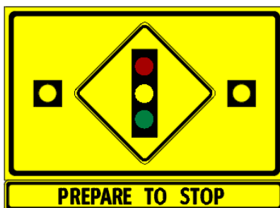
Figure 17: City of Vancouver Advance Warning Flasher (AWF)
