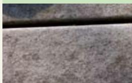
Plastic from consumers and the automotive industry is collected, melted, and formed into 4"x4"x8' (10cm x 10cm x 2.5m), 6"x6"x8'(15cm x 15cm x 2.5m) and larger sizes. This rot-proof material can be left in direct contact with soil.
