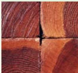
The most common landscape timbers are pressure treated (injected with rot- and insect-inhibiting chemicals under pressure). For years, treatment with chromium copper arsenate was standard (see the Decking table on page 10 for a description of the hazards of this type of wood treatment). Naturally rot-resistant species, such as juniper, can endure ground contact without the application of toxic wood preservatives.
