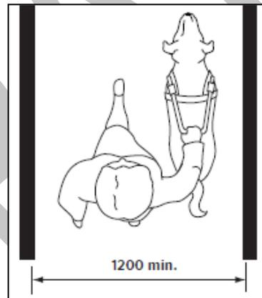
Figure 13: Walkway width (in mm) for persons with a guide dog (CAN/CSA-B651)
