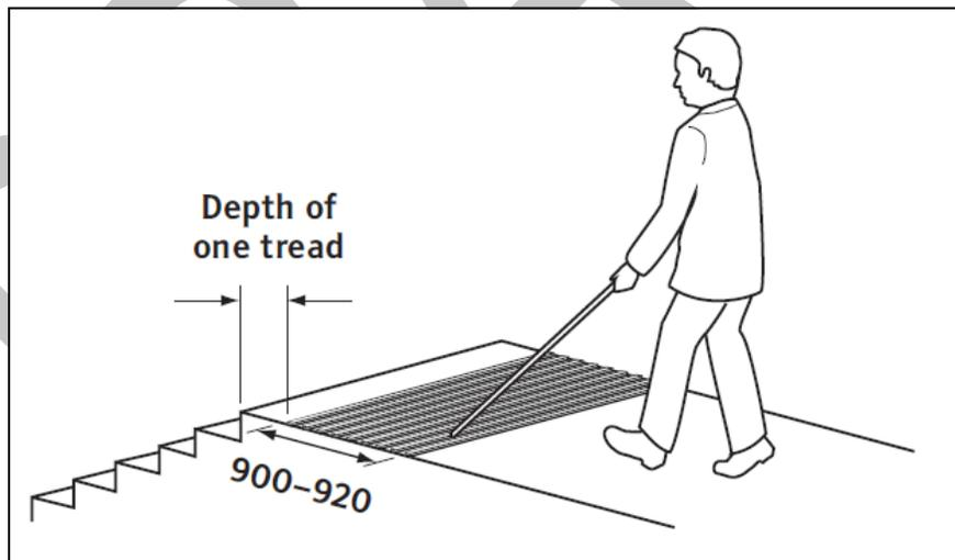
**Figure 25: Detectable Warning Indicator Surface (CAN/CSA-B651)**
