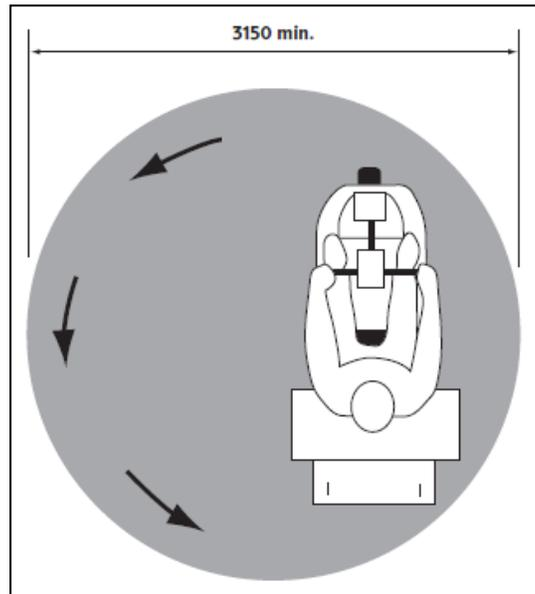
Figure 8: Turning area (in mm) for a person using a large scooter (CAN/CSA-B651)
