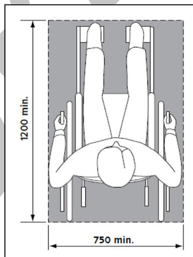
Figure 3: Minimum floor area (in mm) for a person using a manual wheelchair (CAN/CSA-B651)
