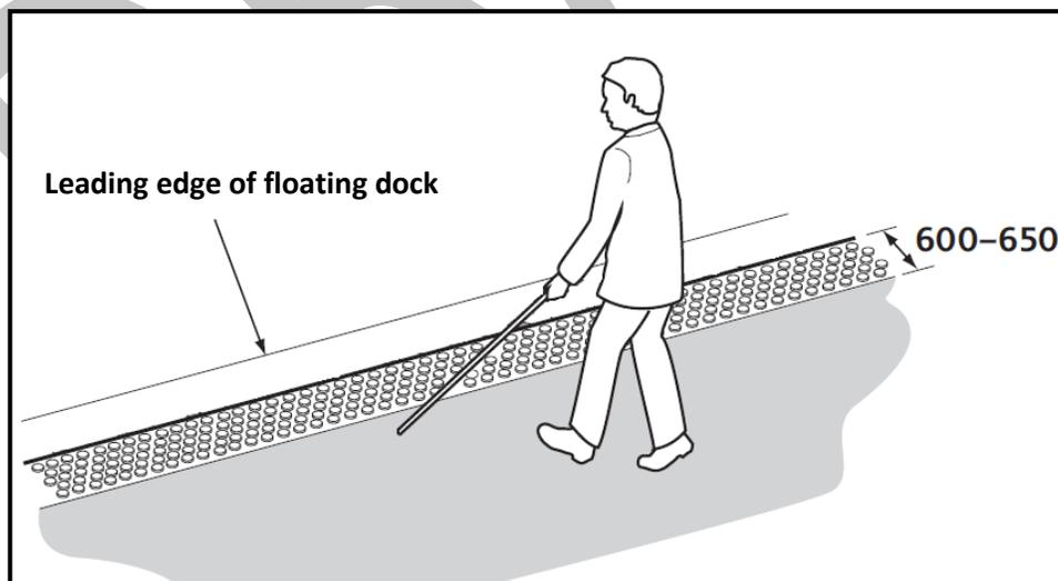
Figure 22: Detectable Hazard Indicator Surface (CAN/CSA-B651)
