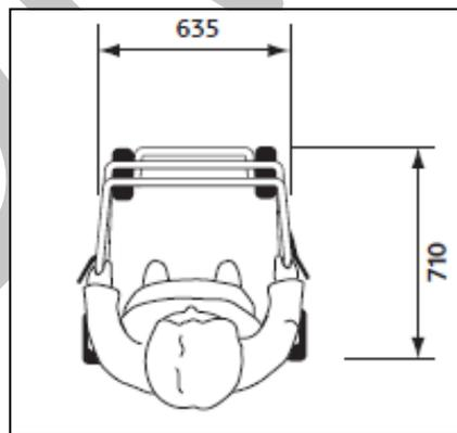
**Figure 5: Floor area (in mm) for a person using a walker (CAN/CSA-B651)**
