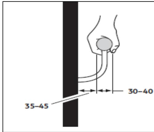
Figure 18: Handrails (CAN/CSA-B651)
