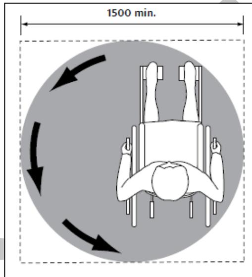
**Figure 6: Turning area (in mm) for a person using a manual wheelchair (CAN/CSA-B651)**
