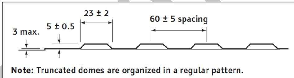
Figure 23: Detectable Hazard Indicator Surface Configuration (CAN/CSA-B651)
