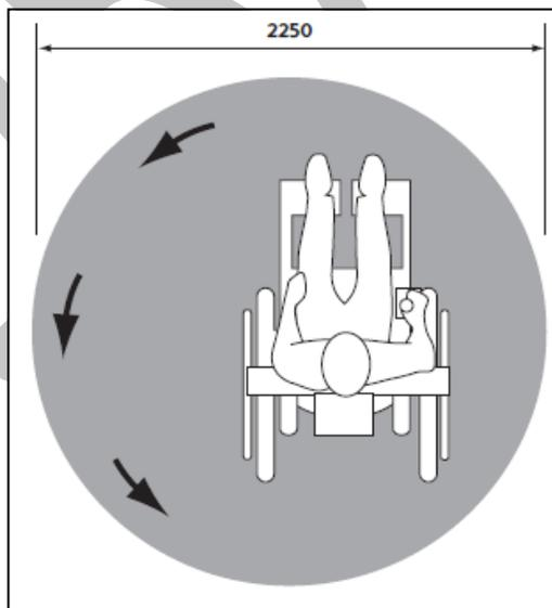
**Figure 7: Turning area (in mm) for a person using a power wheelchair (CAN/CSA-B651)**
