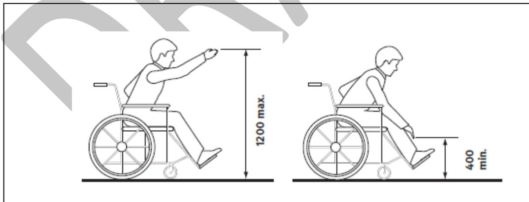
Figure 9: Forward Reach Without Obstruction (CAN/CSA-B651)
