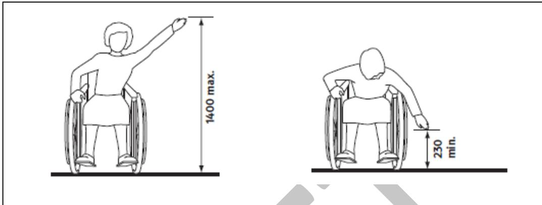
Figure 10: Forward Reach Without Obstruction (CAN/CSA-B651)
