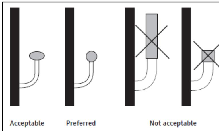
Figure 21: Handrail Shapes (CAN/CSA-B651)
