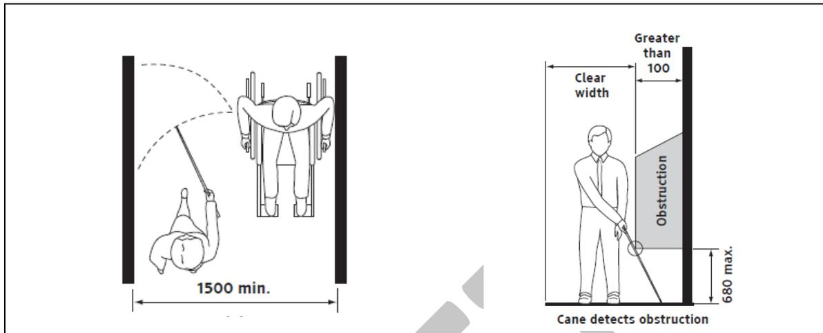
Figure 12: Detection space (in mm) for persons using a long white cane (CAN/CSA-B651)
