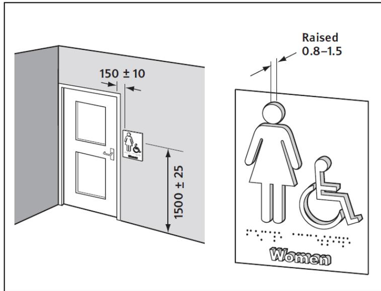
Figure 28: Location and Size of Tactile Signs (CAN/CSA-B651)
