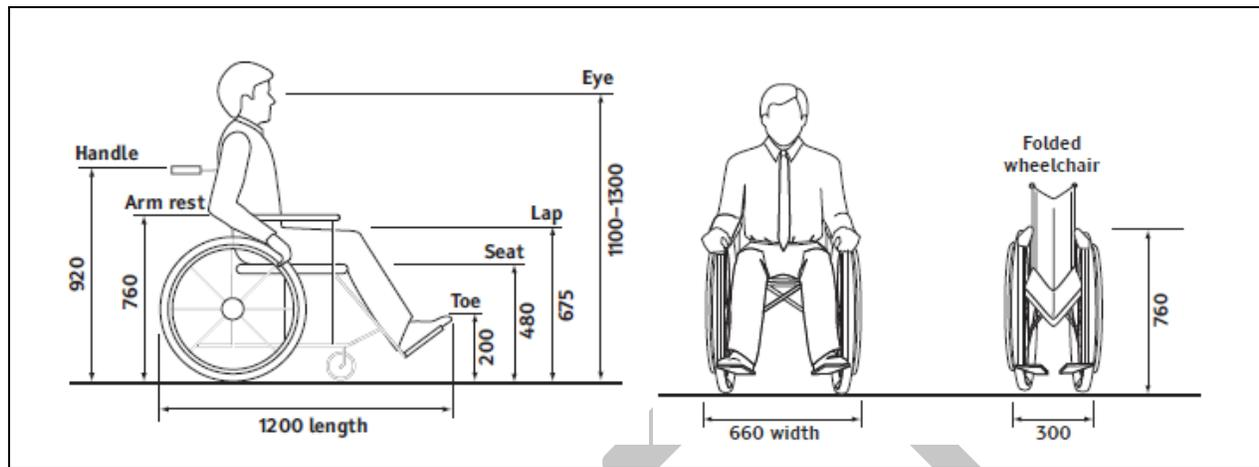
Figure 2: Typical Dimensions (in mm) of an adult manual wheelchair (CAN/CSA-B651)
