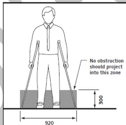
Figure 11: Walkway width (in mm) for persons using crutches (CAN/CSA-B651)
