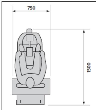
**Figure 4: Minimum floor area (in mm) for a person using a power wheelchair/scooter (CAN/CSA-B651)**
